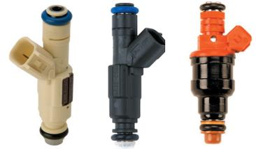
The nominal injection pressure for most Ford EFI systems is 39.15psi (270kPa) “across the injector.” The term “across the injector” takes manifold pressure and fuel rail pressure into account, and is usually referred to as “delta pressure.” (See “Measuring Fuel Pressure” below for more details.) Ford Racing’s fuel injectors are always rated at 39.15psi delta, so the fuel injector sizing discussions found below will assume a fuel pressure of at least 39.15psi delta.
