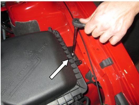
**STEP 10:** Remove 2 screws from the mass airflow sensor and remove from the production intake tube.
