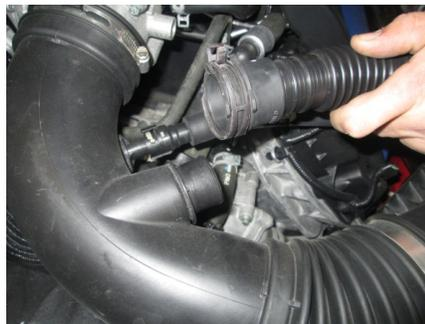
**STEP 4:** Remove bolt holding resonator tube to the frame rail. Remove tube from the bulkhead by pulling gently.
