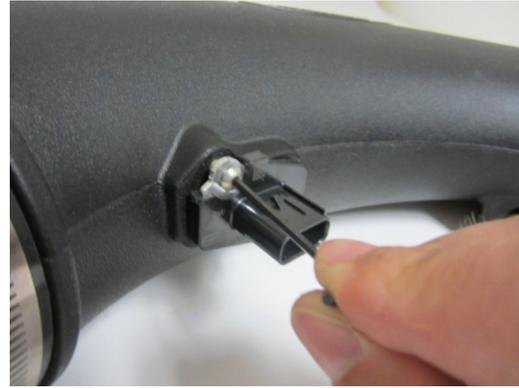
**STEP 12:** Install the provided grommet into the provision on the intake tube. Install the aluminum fitting into the grommet. A small amount of white lithium grease on the aluminum fitting will aid in the installation of the fitting.
