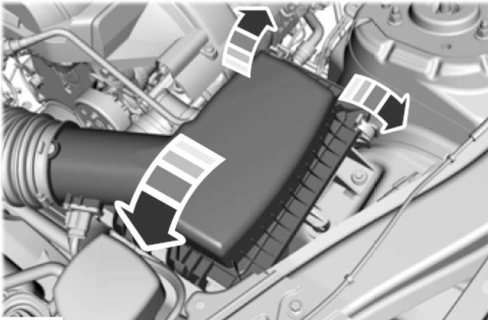
1. Release the two clamps that secure the air filter housing cover.
