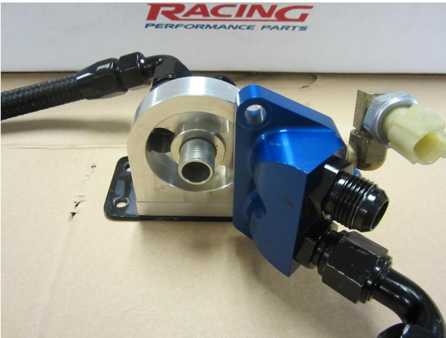
This picture shows the line attached to block adapter port "B" out to oil filter outside holes.
