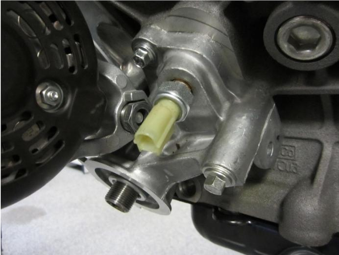
Check and note oil level on dipstick. With oil filter installed and full of oil, remove oil pressure sending unit. Using proper adapters, attach engine pre-lube tank to the port that the sending unit was screwed into. Following the engine pre-lube tank manufacturer's instructions, prime the engine.
