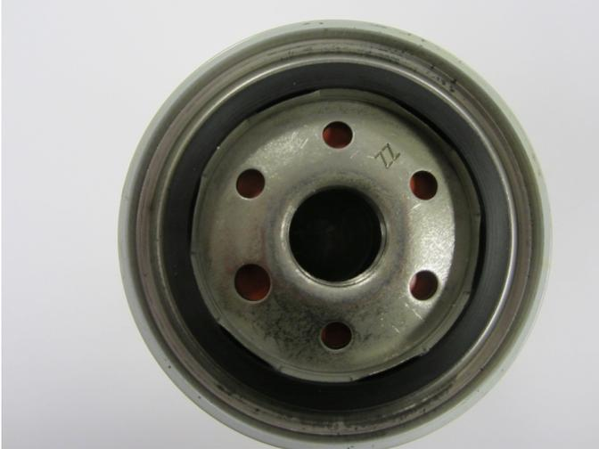
Center opening of the oil filter to block adapter port "A". Oil exits out of the oil filter from the center opening.
