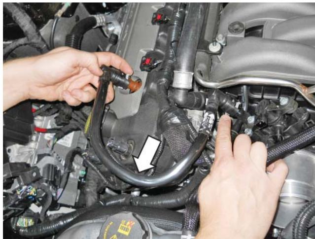
25. Disconnect the fuel supply hose from the fuel rail.
