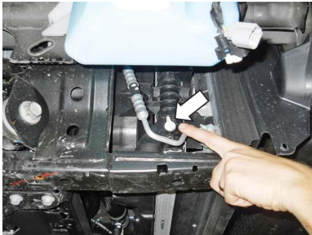
10. If equipped, remove the four (4) nuts and the strut tower cross brace (15 mm socket). The strut tower cross brace cannot be reused after the supercharger has been installed. Discard the nuts.
