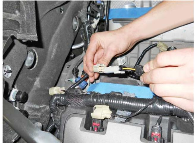
3. Route the extension wiring harness to the RH side cylinder head.
