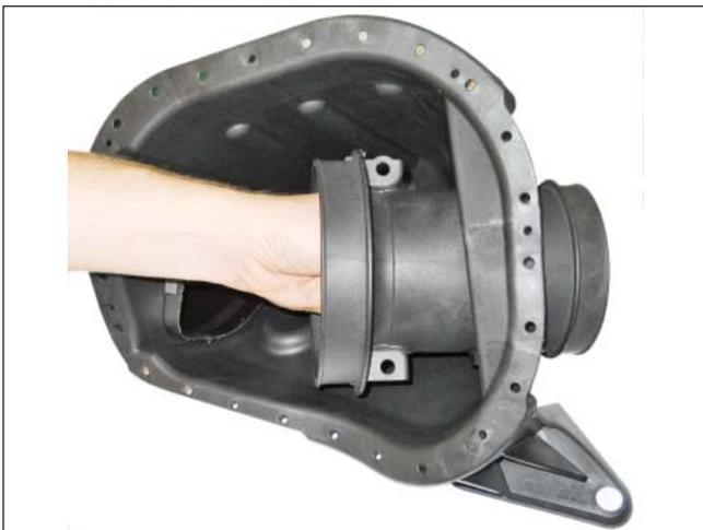
4. Align the holes on the MAF tube assembly with the J-Clips on the airbox tray. Install two (2) Bolts (W500224) (M8 X 25) from Hardware Kit A (1315-TVSHKA) and torque to 10 Nm (10 mm socket).
