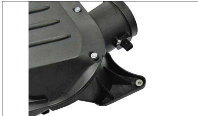
10. Remove the rubber mounting isolator from the bottom of the factory airbox and install it onto the mount on the bottom of the new airbox in the same orientation.
