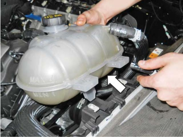
44. Disconnect the clamp on the end of the upper radiator hose at the radiator. Use a rag to catch excess coolant. On the thermostat housing end of the hose, push the clip down on the connector and remove the upper radiator hose from the vehicle.
