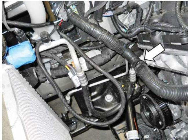
9. Route the intercooler pump wire harness over the top and in front of the wiper washer bottle. Secure it in place with zip ties as necessary.
