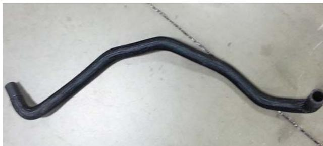
Intercooler pump inlet hose (1315-8D029)
