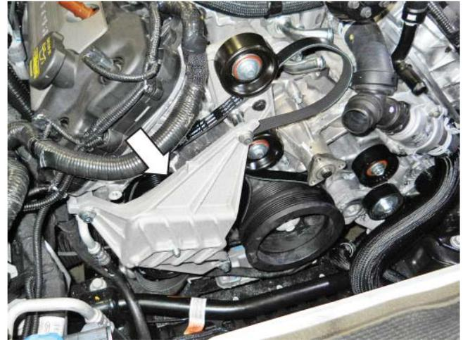
10. Install one (1) M8 x 1.25 x 41 mm Bolt (W705128) found in Hardware Kit C (1315-TVSHKC), to fasten the Tensioner Bracket to the Upper FEAD Bracket. Torque all three (3) Tensioner Bracket bolts to 25 Nm.
