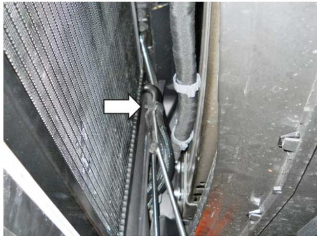
11. Install the hose onto the intake manifold inlet and secure it with the Clamp (CT19X12) from Hardware Kit G (1315-TVSHKG).
