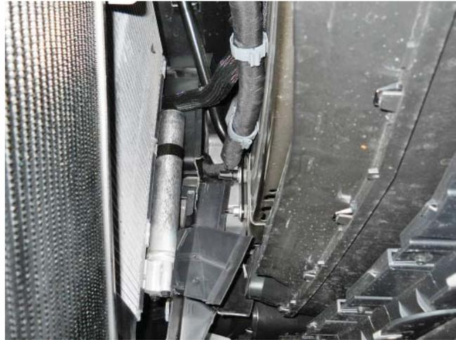
7. Reinstall the hose onto the LTR outlet, and recheck the hose fit. Adjust as necessary until the hose passes through the close-out panel without being kinked.
