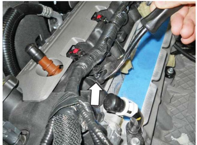
2. Peel back the insulation at the base of the ground wire that was attached to the stud on the front cover. Trim back part of the insulation until the ground wire is exposed.
