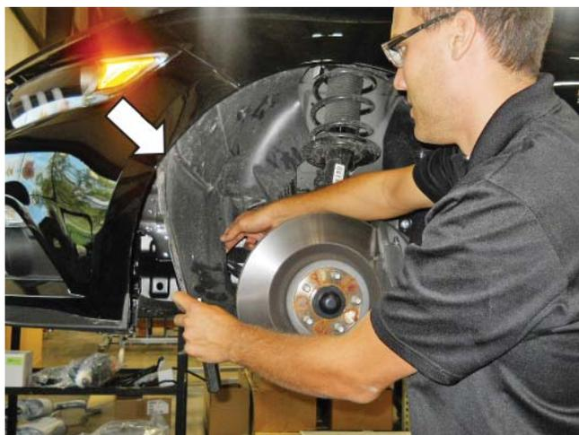
8. Remove the nineteen (19) lower close-out panel bolts and the two (2) pushpins. Remove the lower close-out panel from the vehicle (7 mm socket).
