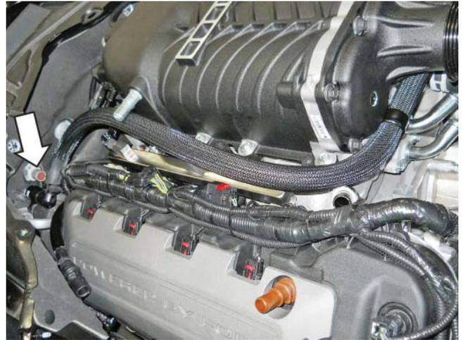
27. Install the heater hose connector to the bottom port (heater outlet) at the RH firewall.
