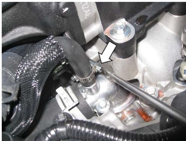
7. Install the other end of the hose to the engine degas bottle as shown. Secure the constant tension clamp.
