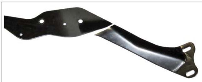
3. Use a suitable tool to file the sharp end where the brace was cut.
