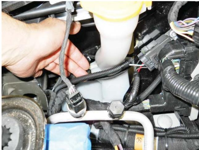
10. Zip tie the excess harness out of the way and secure it to a safe location.
