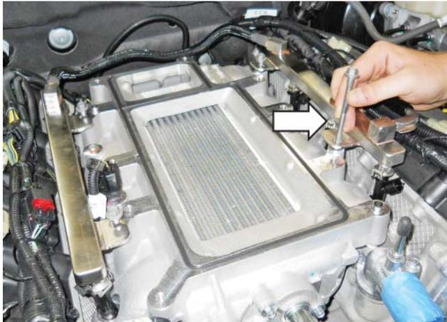
8. Connect the eight (8) fuel injector electrical connectors.
