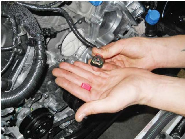
3. Populate the new connector such that the yellow with violet wire is in position 1, the blue with green wire is in position 2, the brown wire is in position 3, the blue with orange wire is in position 4, the yellow wire is in position 5 and the green with violet wire is in position 6. Install the red plastic lock into the connector to secure the wires in place.
