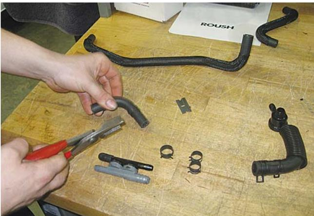
9. Install the aspirator to brake booster line (1315-9D690) into the black port on the brake aspirator assembly. Then install the check valve that plugs into the brake booster.
