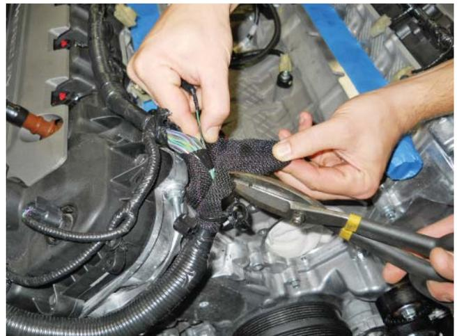
3. Separate the ground wire further back into the harness. This will create slack necessary for relocating the ground.
