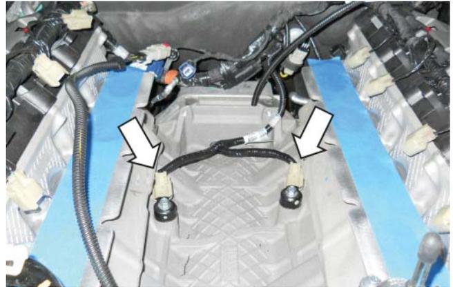
5. Reinstall the convolute and rewrap the wires with electrical tape as required.
