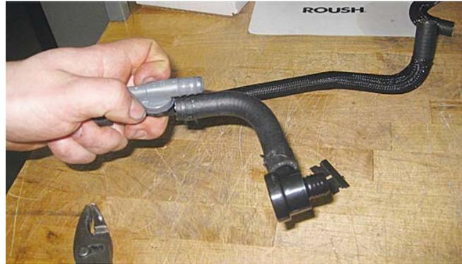
10. Install the line that goes from the supercharger to the aspirator assembly (1315-9D692) into the 1/2-inch grey fitting on the aspirator assembly.
