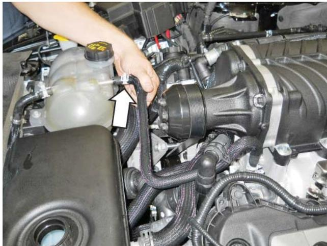
8. Ensure that all intercooler hoses, the degas hose and all clamps and wiring have been installed to provide maximum clearance to the supercharger belt.
