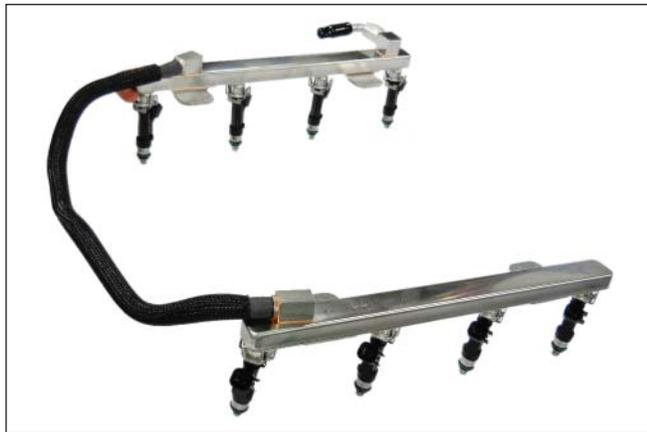
2. Apply assembly lube to the injector O-rings and install the injectors into the new Fuel Rail (1315-19F792).
