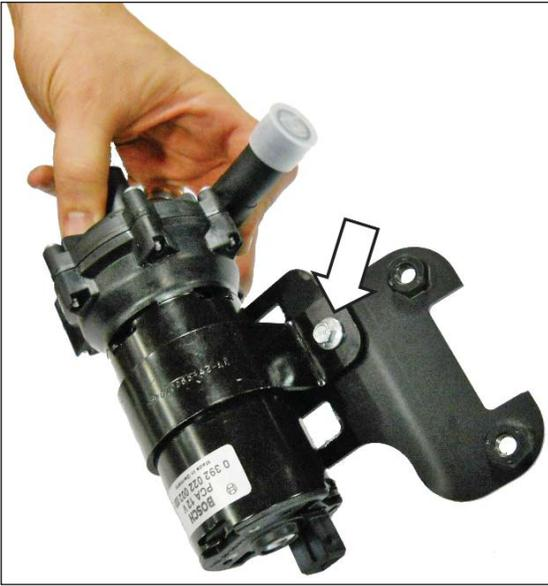
4. Place the intercooler pump assembly and bracket in mounting position with the pump in-board to the vehicle. Install two (2) Bolts (W500224) (M8 x 25) into the weld nuts. Torque to 25 Nm.
