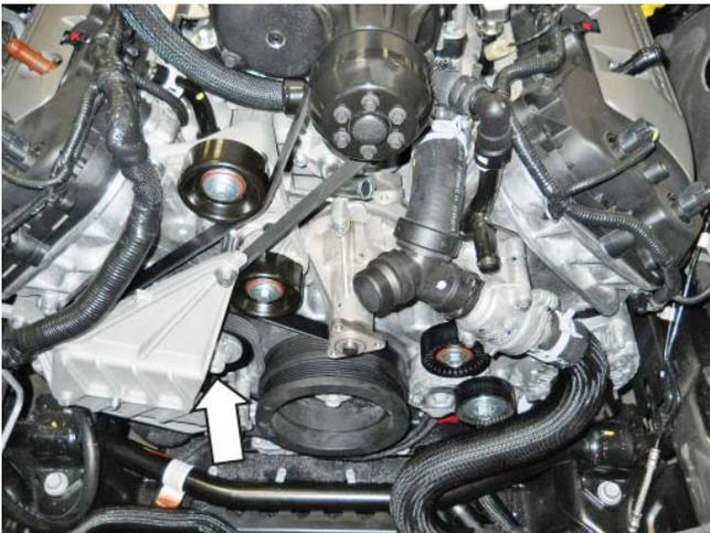
12. Re-install the water pump pulley using the three (3) removed bolts. Torque the bolts to 25 Nm.
