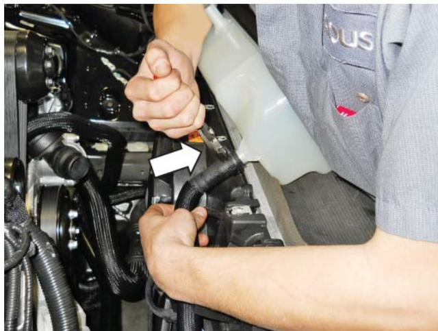
3. Ensure that the Clip (20860) installed during the electric fan modification is in place at the bottom of the Intercooler Degas Bottle (1315-8D080).
