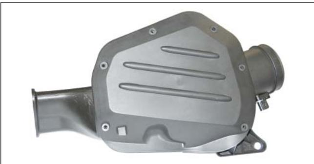
9. Remove the grommets and sleeves from the factory lower airbox. Install the grommets and sleeves onto the new airbox assembly.
