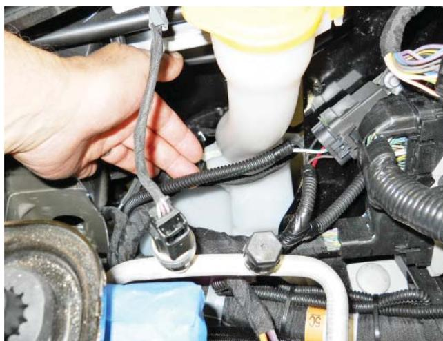
9. Retain the engine harness to the front cover using the zip tie with fur tree (156-00329) found in Hardware Kit E (1315-TVSHKE).
