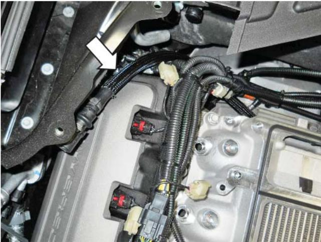
6. Connect the ACT sensor from ACT Harness (1315-12A690) to the intake manifold.
