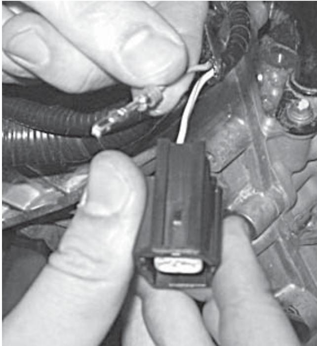
3. Connect the Evaporative Emissions Canister Purge Valve Extension Harness (13119G866) to the newly installed connector. The wire colors on each side of the connector pair should align. Route the harness along the main wiring harness to the rear of the passenger side cam cover. Use tape or zip ties to secure the extension harness to the main harness.
