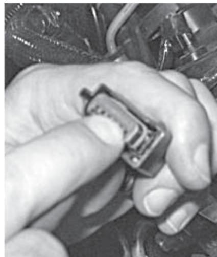
4. Connect the TPS/ETC Extension Harness (131114A595) from Hardware Kit E (1315-TVSHKE) to the newly installed connector. The wire colors on each side of the connector pair should align. Route the harness along the main wiring harness to the rear of the driver side cam cover. Use tape or zip ties to secure the extension harness to the main harness.
