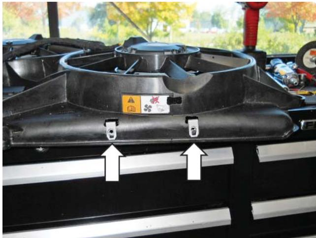
4. Insert the Clip (20860) found in Hardware Kit H (1315-TVSHKH) onto the tab on the bottom of the Intercooler Degas Bottle (1315-8D080).
