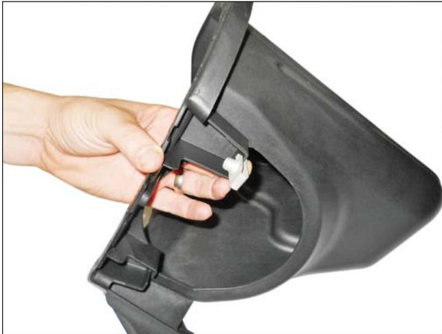
3. Place the MAF Tube Assembly (1315-12B579HC) through the opening of the airbox tray from the inside.
