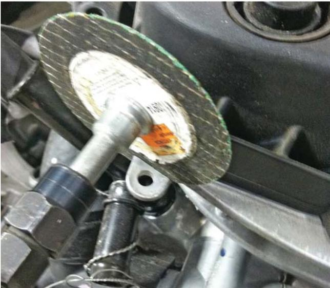
5. Using a suitable cutting tool, remove the mounting tab. Follow the edge of the part. Use caution as to not contact the cam covers.
