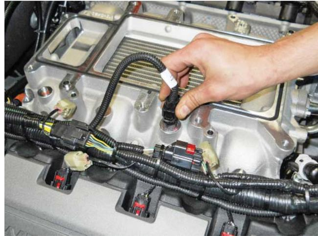
7. Lube the lower fuel injector O-rings with assembly lube. Install the fuel rail and injectors into the intake manifold. Be sure each injector is properly seated into the intake manifold. Install the previously removed fuel rail mounting bolts. Tighten the fasteners in two stages with the sequence shown. Stage 1; torque bolts to 10 Nm. Stage 2; tighten bolts an additional 45 degrees.
