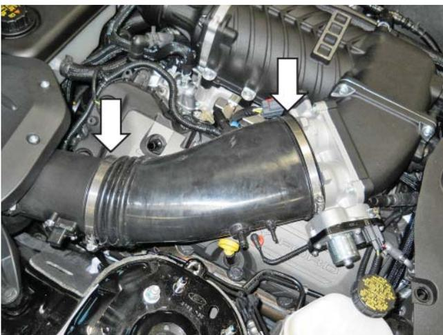
6. Install the PCV Fresh Air Inlet Tube (1315-6758) by connecting the 90-degree fitting to the driver side cam cover and angled fitting to the PCV fitting in the clean air tube.
