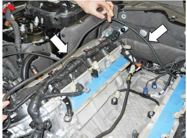
5. Install the intercooler pump harness red power wire to the first post in the fuse box. Tighten the nut to 10 Nm.
