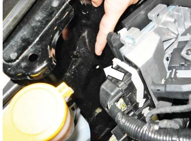
2. Install the relay and fuse from the Intercooler Pump Wiring Harness (1315-8W501) through the hole and secure it with one (1) M6 x 14 Bolt (N605771) and one (1) M6 Nut (W520412). These parts can be found in Hardware Kit E (1315-TVSHKE).
