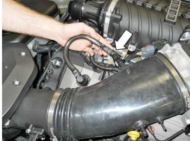
7. Route the MAF wire harness around the airbox assembly and connect the harness to the MAF sensor. Make sure the red lock is engaged on the connector.
