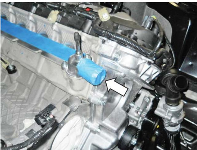
58. Tape off and block the thermostat housing ports.
