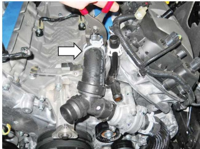
52. Remove the two (2) bolts from the thermostat housing (8 mm socket).
