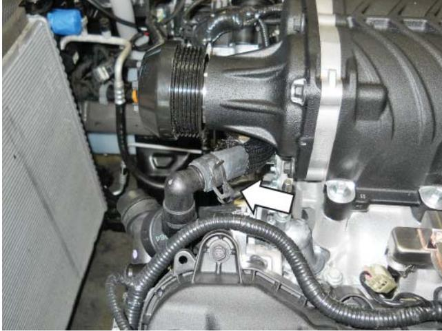
25. Route the line around the front of the engine underneath the snout of the supercharger towards the heater core. Remove the top intercooler tube bolt and install the P-clamp tab using the fastener on the intercooler coolant inlet.
