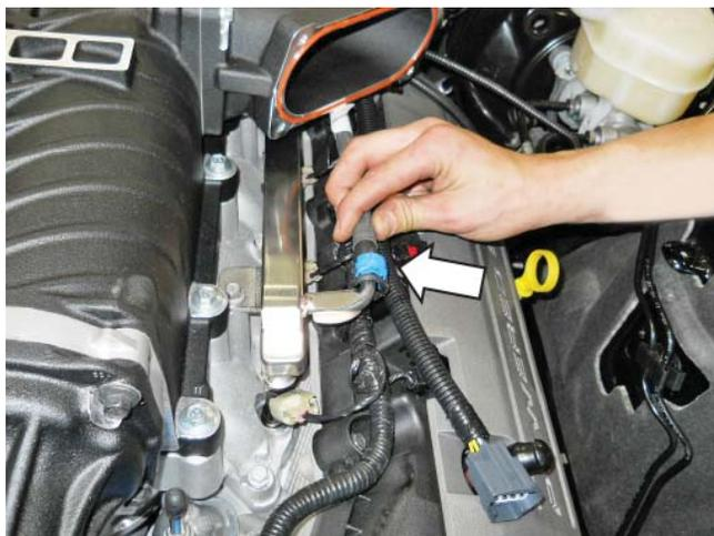
19. Install the Throttle Body Assembly (R07060150) on the throttle body spacer. Use four (4) M6 x 32.5 mm Bolts (R18020009) found in Hardware Kit B (1315-TVSHKB) to secure the throttle body assembly to the spacer. Torque bolts to 10 Nm.
