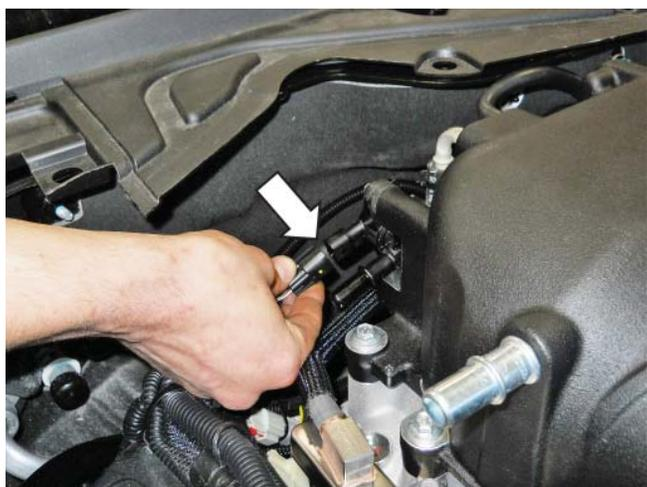
22. Install the Evaporative Emission Canister Purge Valve Line to the body line tube below the brake booster. Slide the green clip to lock the connector. Route the rest of the line behind the cylinder head to the RH rear of the supercharger.
