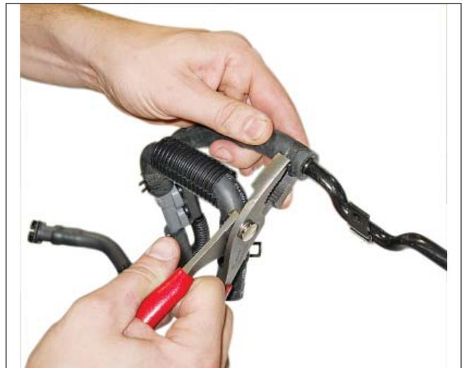
7. Use the supplied brake aspirator plug (CS2575) to plug the black port that is diagonal to the 1/2-inch grey port of the aspirator assembly. (The arrow indicates the 1/2 inch grey port.)
