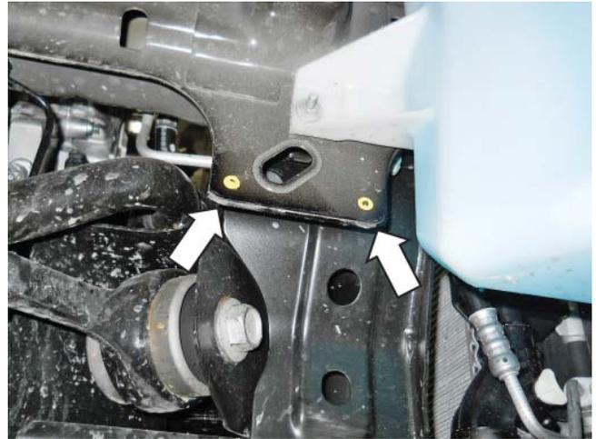
2. Start by drilling two (2) pilot holes. Then, drill out two (2) 3/8" holes.
