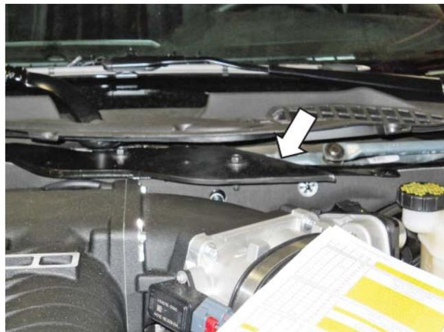
2. Install the nuts on the studs and torque to 25 Nm using a 15 mm socket.
