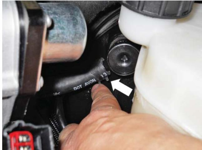
12. Install the brake aspirator hose assembly. Connect the hose (with 1/2" barbed fitting) from the supercharger to the 1/2" brake line and secure it with the attached clamp.
