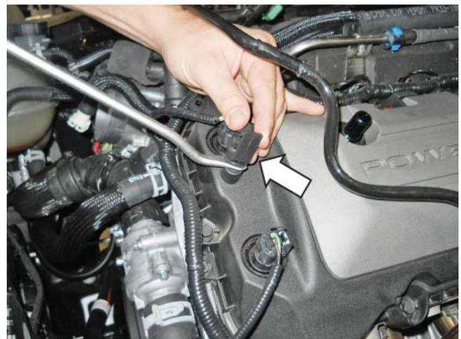
Remove retainer on cam cover
