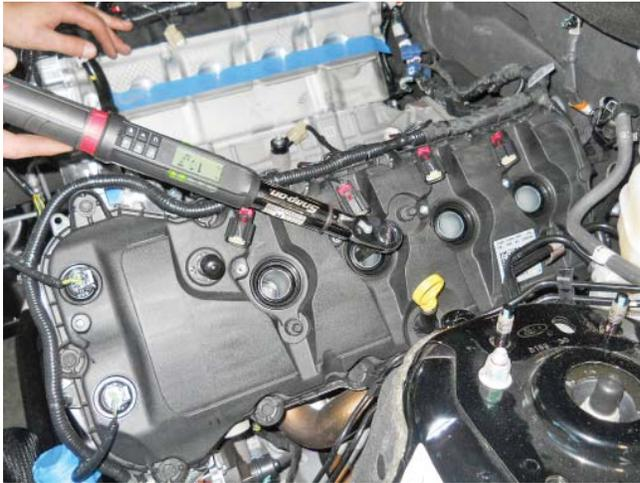
8. Apply a small amount of dielectric grease to the inside of the coil on plug boots before attaching to the spark plugs. Install the ignition coil on plugs in their original position. Install the coil on plug bolts and torque to 6 Nm.
