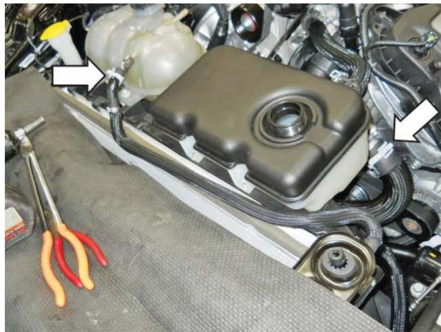
5. Transfer the hose clamp from the bottle end of the factory degas hose to new 3/8" Engine Degas Hose (1315-8276). Install the hose clamp (62002) onto the other end of the engine degas hose.
