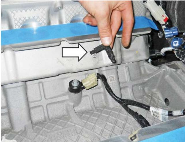
2. Loosen the two (2) bolts which retain the knock sensors to the engine block (10 mm socket). If necessary, one (1) of the bolts and sensors can be removed for this modification process.
