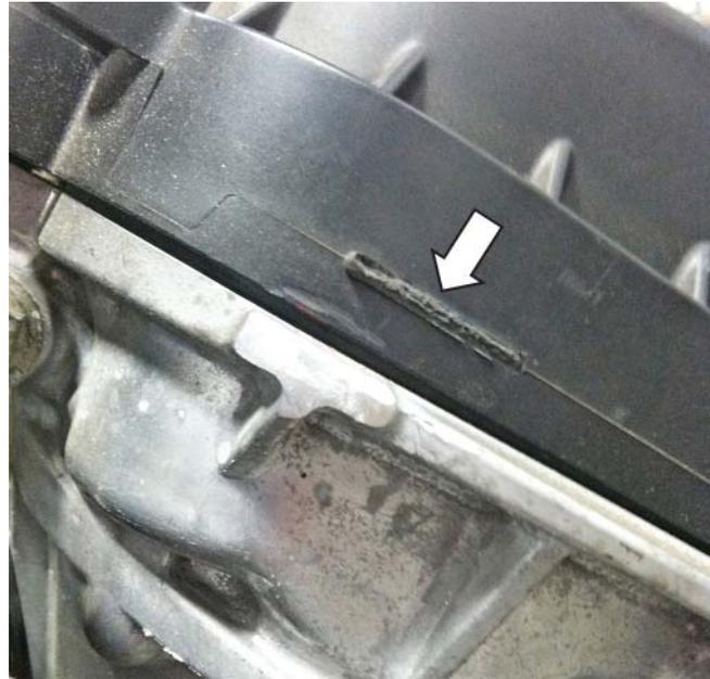
6. Deburr any rough edges on the cover and remove the retention harness from the wire harness.
