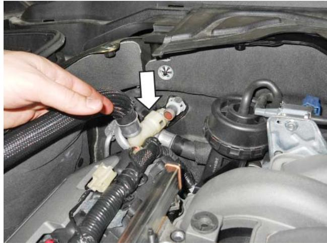
33. Disconnect the heater feed and return hoses located at the front of both the LH and RH cylinder head intake flanges. Disconnect and remove the hoses from the ports on the RH firewall.
