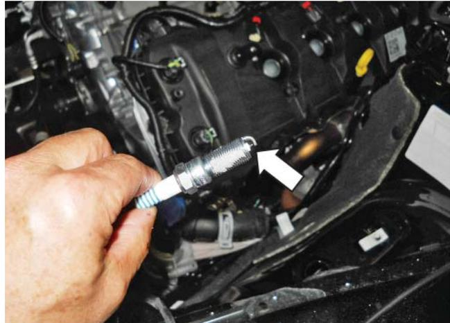
7. Install the new spark plugs using a 5/8" spark plug socket and 6" extension. Torque to 14 Nm.
