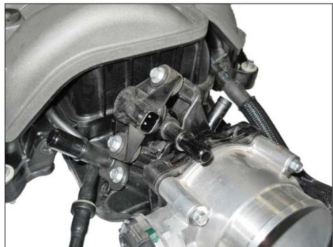
2. Install the valve into the rear of the supercharger (1315-6F066) using two (2) M6 x 1.0 x 35.5mm Bolts (N808429) found in Hardware Kit B (1315-TVSHKB). Torque bolts to 8-12 Nm.
