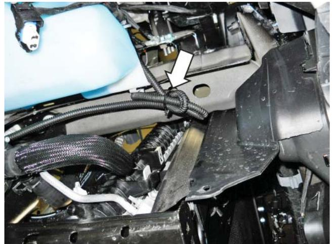
**NOTE:** Route all intercooler hoses very carefully. It is critical for intercooler performance that these hoses are not kinked once installed into the vehicle.
