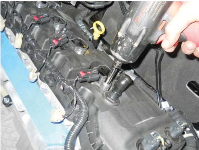
4. Remove the coil on plug assemblies and label them so they can be reinstalled in their original position. A slight twisting motion will break the seal and ease removal.
