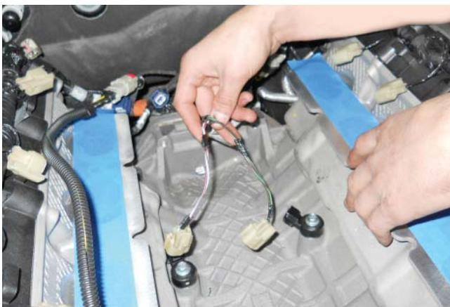
4. Temporarily fit the sensors as follows to determine where to rewrap the wires. Install and rotate the
