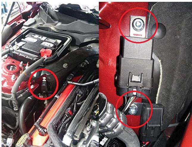
2. Apply blue Loctite (or equivalent) to two (2) M6 nuts (W520412) and secure to the studs.
