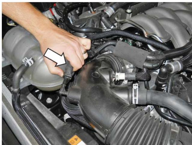
15. Disconnect the vacuum line from the air cleaner tube.
