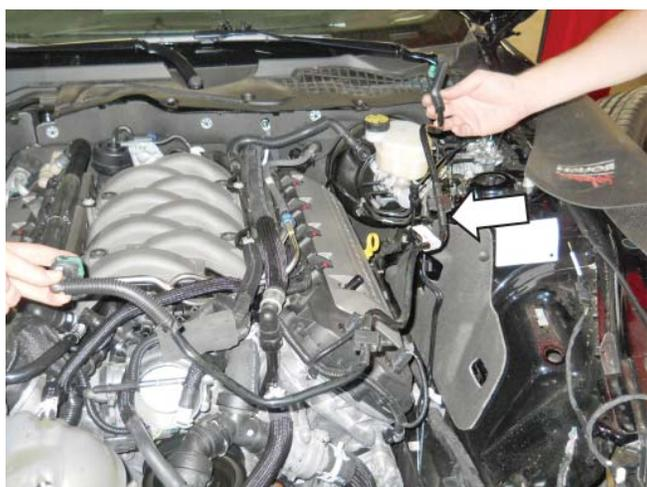
24. Remove the PCV Purge line from the intake manifold and RH cam cover. This line will not be reused.
