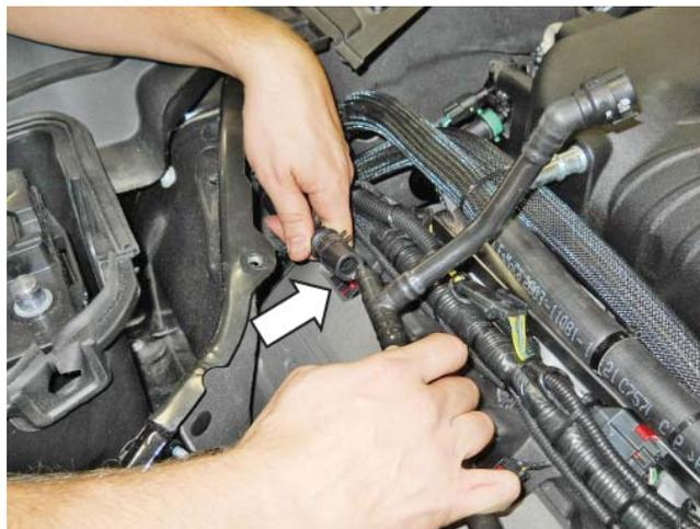
32. Connect the PCV Purge Line (13116K817) to the PCV Valve on the RH cam cover and the port on the RH side of the supercharger.
