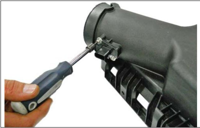
7. Transfer and install the factory MAF sensor into the MAF tube assembly using the original MAF sensor bolts (M4 X 0.7 X 10) and tighten with a T-20 Torx bit. Torque the screws to 1.8–2.2 Nm. Be careful not to over tighten these screws. Wiggle the MAF sensor to ensure that it is properly fastened.
