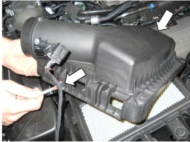
20. Remove the filter from the airbox. Remove the mounting bolt at the side of the airbox (10 mm socket). Pull up and remove the lower airbox from the vehicle.
