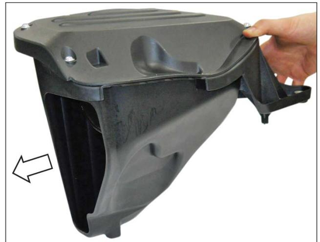
4. Secure the airbox using the M6 bolt from the original airbox and torque to 10 Nm.
