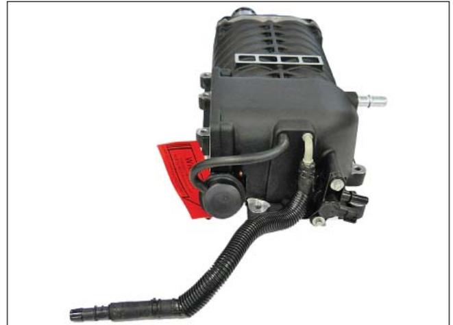
5. Connect the Supercharger Bypass Reference Vacuum Line (7R3V-9E498) to the bottom fitting on the supercharger bypass actuator.
