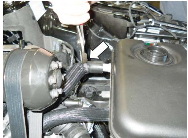
10. Install the hose to the intercooler cooler outlet using (1) Clamp (CT19X12) from Hardware Kit G (1315-TVSHKG).
