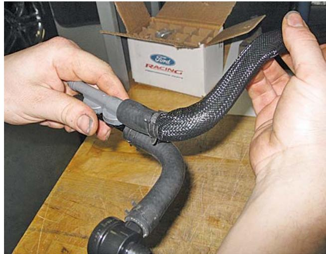
11. Install the hose that goes to the clean air tube (1315-9D691) into the remaining port on the brake aspirator assembly.
