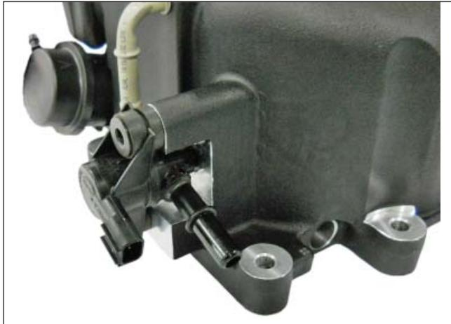
3. Connect the Supercharger Boost Bypass Actuator Hose (1315-9E498) found in Hardware Kit D (1315-TVSHKD) to the top port on the actuator and route to the small port on the supercharger.
