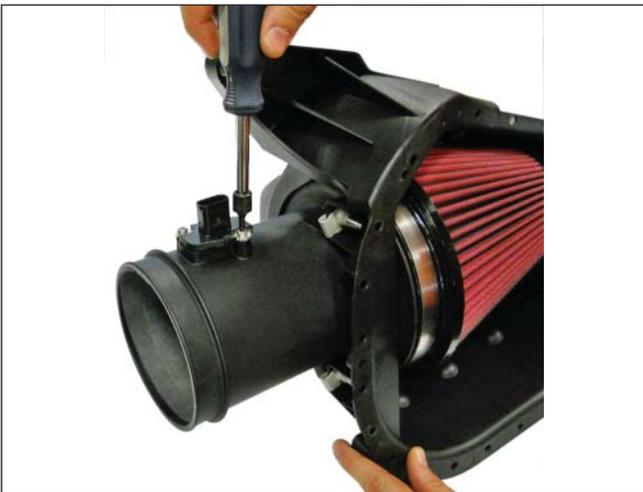
8. Install the Upper Airbox Cover (1315-9643) on the airbox tray. Using a T-30 Torx head bit, install six (6) Bolts (W506976) from Hardware Kit A (1315-TVSHKA).
