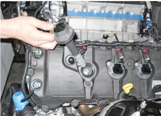
5. Use a 5/8" spark plug socket and 6" extension to remove the eight (8) factory spark plugs and set aside. These will not be re-used.
