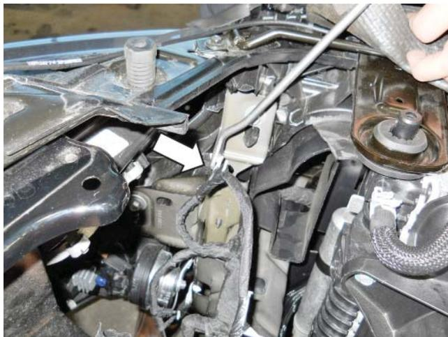
2. Install the Dirty Air Duct (1315-9F763) at the LH side of the radiator.
