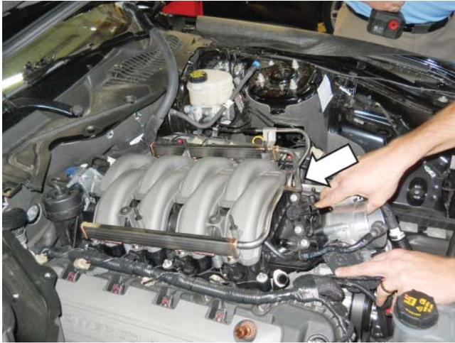
41. Clean the intake mounting surfaces and apply tape over the open intake ports to prevent engine contamination.
