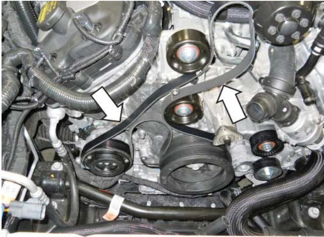
9. Loosely install the FEAD Tensioner Bracket Assembly (13118B603) onto the front cover using two (2) M8 x 1.25 x 120 mm Bolts (N811329) found in Hardware Kit C (1315-TVSHKC).
