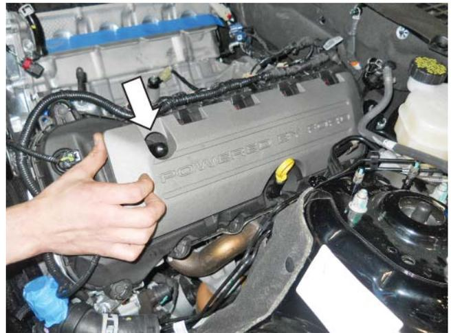
2. Disconnect the electrical connectors for each ignition coil (eight [8] places).
