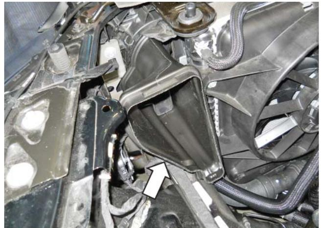
3. Lower the airbox assembly into mounting position. Align the airbox assembly opening with the dirty air duct and press it into the dirty air tube until properly installed. A snap will be heard when properly seated.
