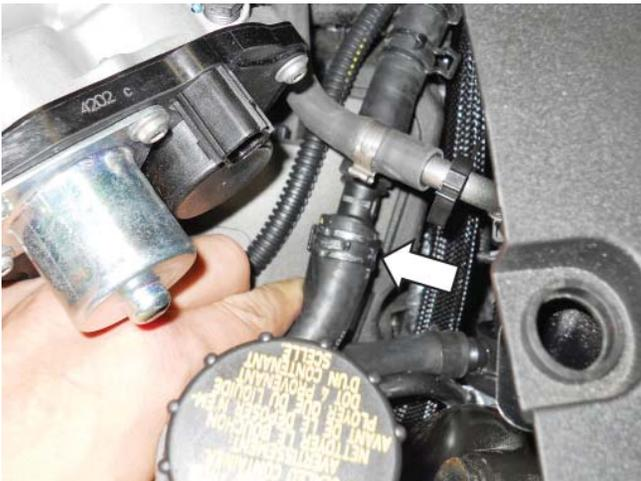
13. Connect the check valve on the brake vacuum and aspirator assembly to the brake booster.
