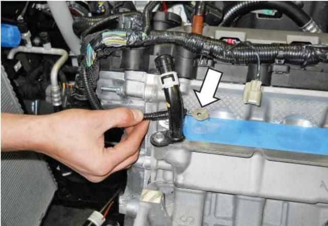
5. Use snips to cut off the bent metal tab on the end of the ground tab.
