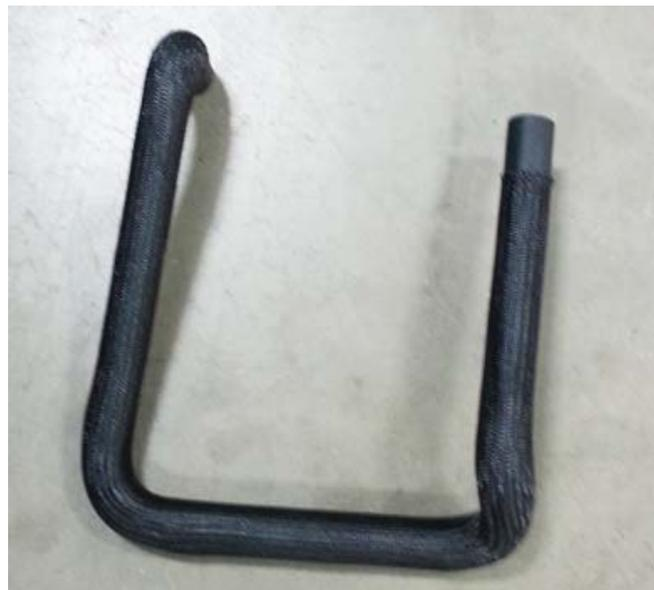
Intercooler pump outlet hose (1315-6K236)
