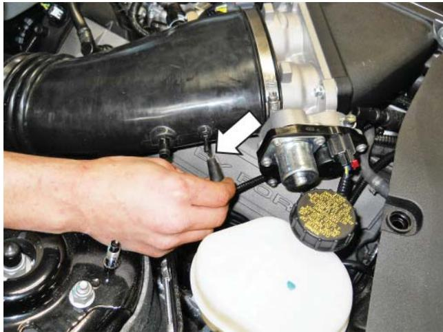
9. Connect the brake aspirator hose assembly (hose 3) to the fitting on the clean air tube.
