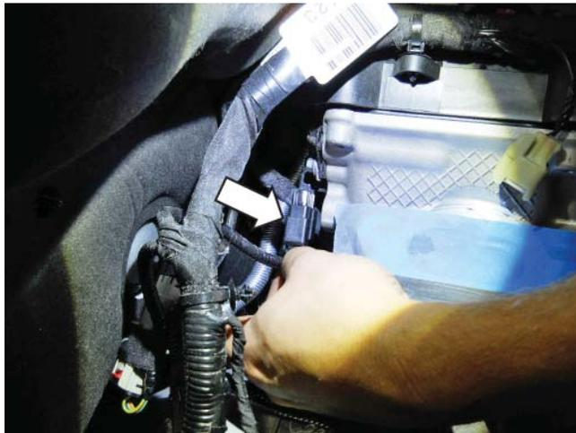
4. Route the intercooler pump wire harness in back of the cylinder head along the RH engine harness to the area near the fuse box.
