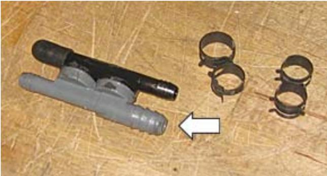
8. Use the takeoff clamps and attach them to the aspirator to brake booster hose (1315-9D690).
