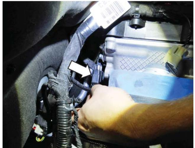
5. Route the intercooler pump wire harness in back of the cylinder head along the RH engine harness to the area near the fuse box.
