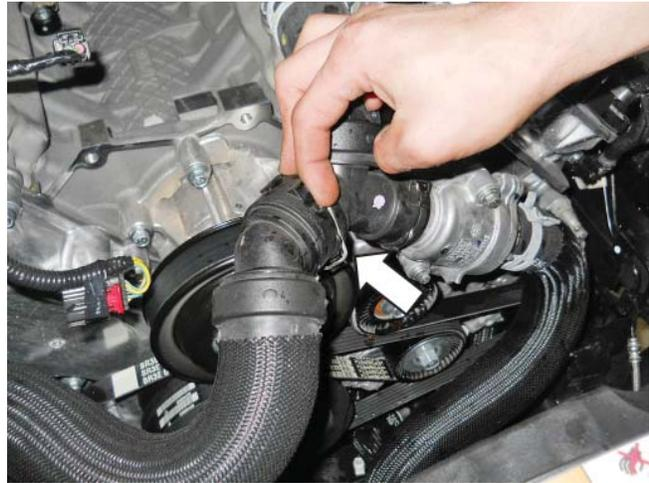
45. Loosen the water pump bolts.
