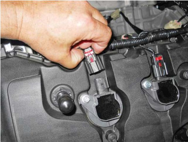
3. Remove the eight (8) fasteners holding the coil on plug assemblies in place (8 mm socket). Save the fasteners for re-use.
