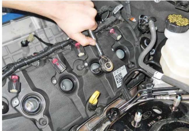
6. Unpack the eight (8) provided Spark Plugs (BL3E-12405) which are pre-gapped to 0.9 mm. Check to ensure the gap is intact and none are damaged.
