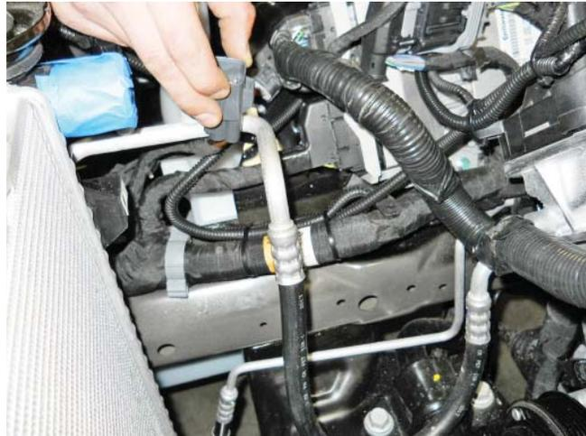
8. Retain the engine harness to the front cover using the zip tie with fur tree (156-00329) found in Hardware Kit E (1315-TVSHKE).
