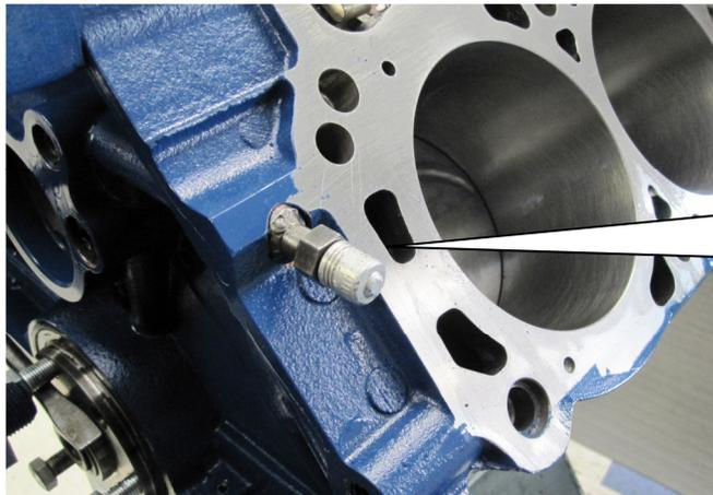
Oil pressure available at the right rear of block via -4 AN fitting with an O-ring seal.
