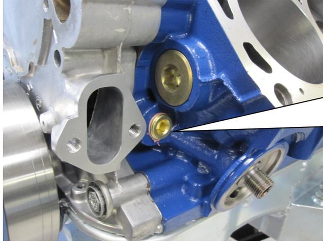
Use caution when tightening 1/2 NPT oil galley plug. **40 Ft. Lbs. MAX.** *Overtightening can cause cracking in this area.*
