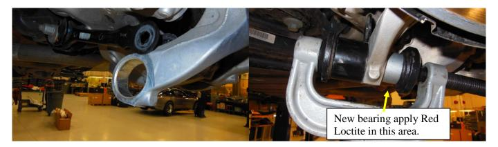
Step 7: Press in new bearing and ensure bearing is centered in knuckle. **Note: Use Red Loctite on bearing mating surface.**
