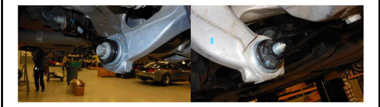
Step 9: Reinstall rear wheels, remove jack stands and lower vehicle.
