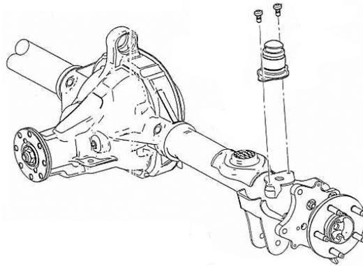
**STEP 4:** Install new Ford Racing jounce bumpers and bolts. Torque bolts to 28 to 32 Nm
