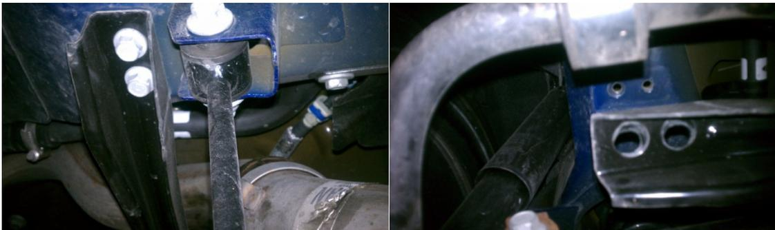
**NOTE:** Lubricate the muffler assembly isolators with soapy water to ease in removal.
