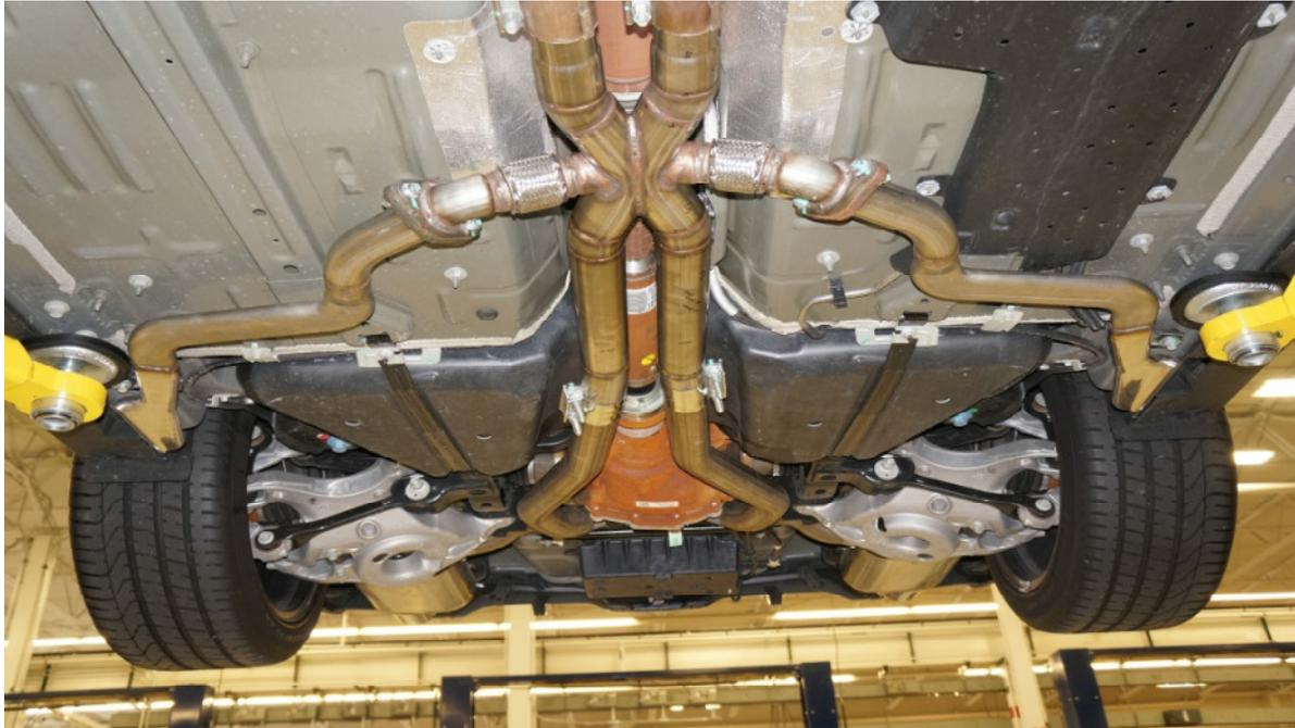
**STEP 11:** Now install supplied bolts into right and left side pipe tips. Torque to 18 lb.ft (25 Nm).
