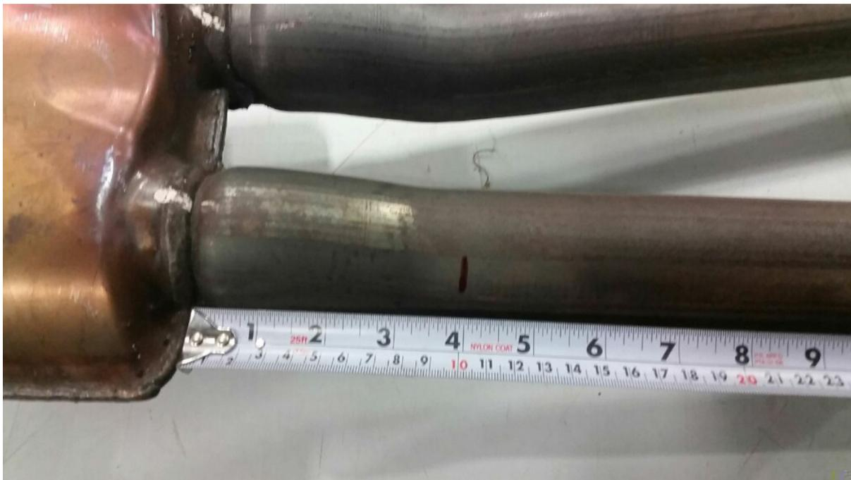
**STEP 6:** Slide the Quad pipe into RH catalytic converter and LH muffler inlet pipe clamps making sure to center the clamps between the two pipes. Snug both clamps to hold Quad pipe in place.
