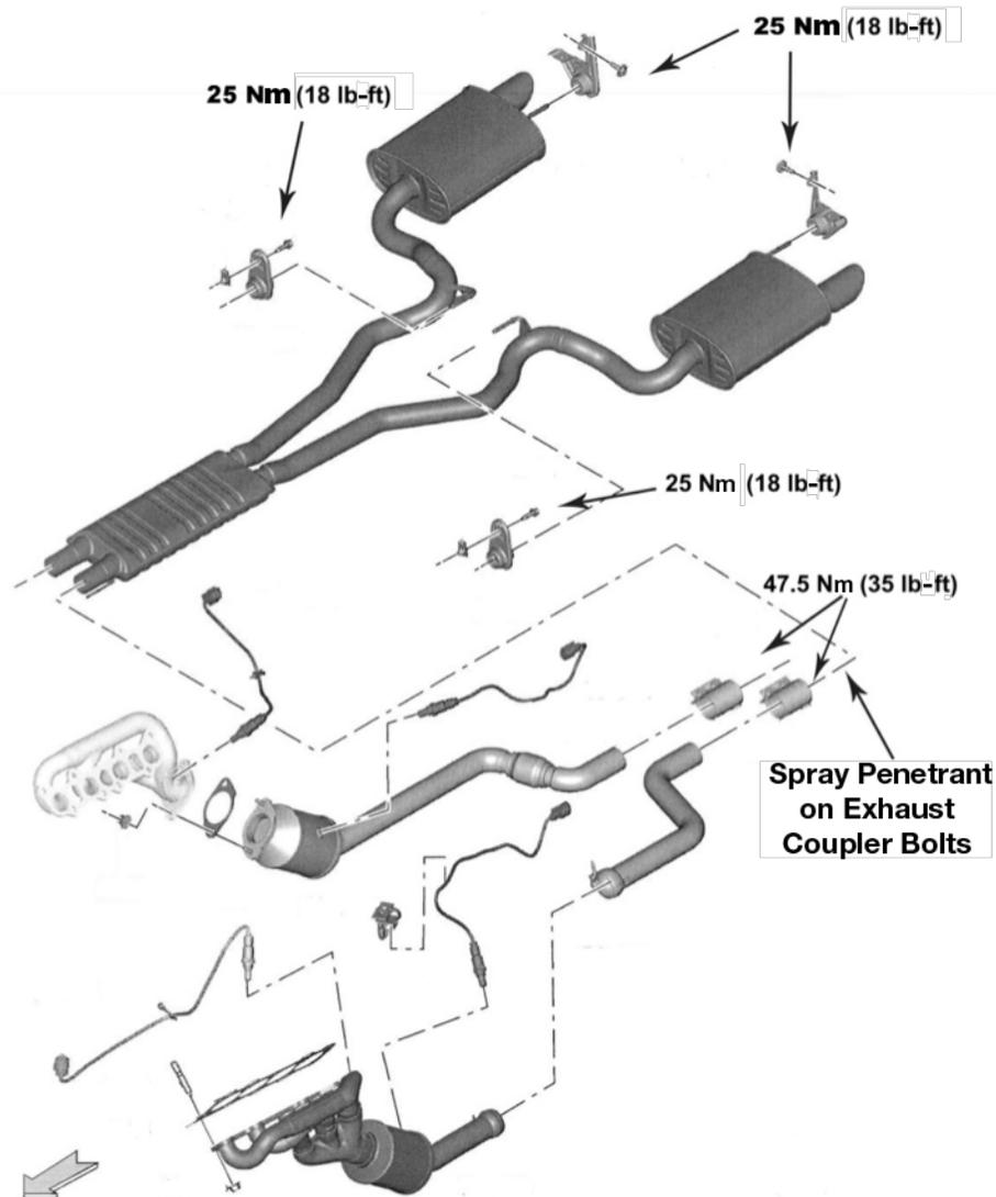
**Step 3:** Using a 15 mm socket, loosen nuts on clamps. (See Fig. 3)
