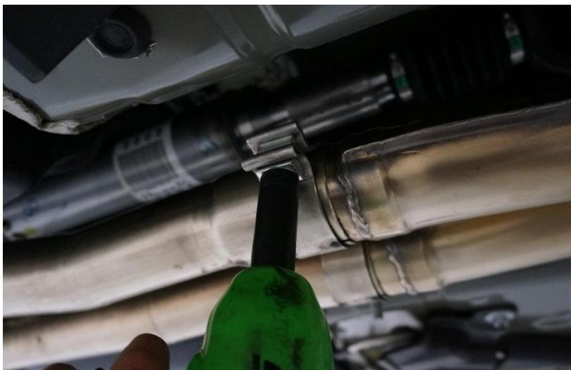
**STEP 4:** Using a 13mm socket remove bolts from exhaust hangers in rear Sub frame.
