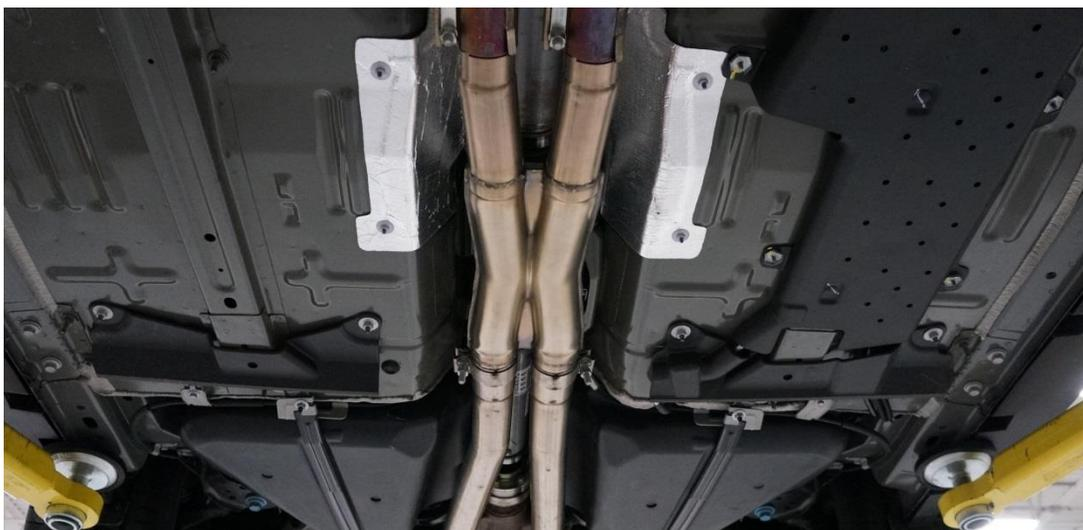
**Step 9:** Install factory removed hangers onto under axle pipes.
