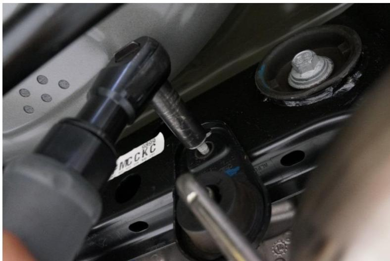
**Step 11:** Using a 13mm socket tighten bolts to 25 nm (18 lb-ft) in rear Sub frame exhaust hangers.
