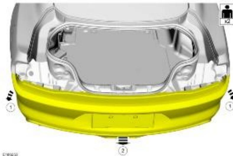
**Step 20:** Disconnect the rear bumper wiring harness electrical connector.
