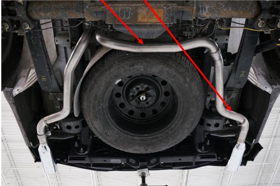
**STEP 11:** Align the right side tail pipe and tip and tighten.
