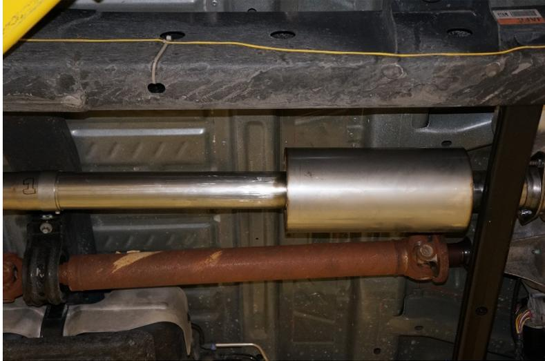
**STEP 2:** Install the proper "Mid Pipe" for your wheel base. Be sure to slip a clamp onto the pipe, clamp to be tightened later.
