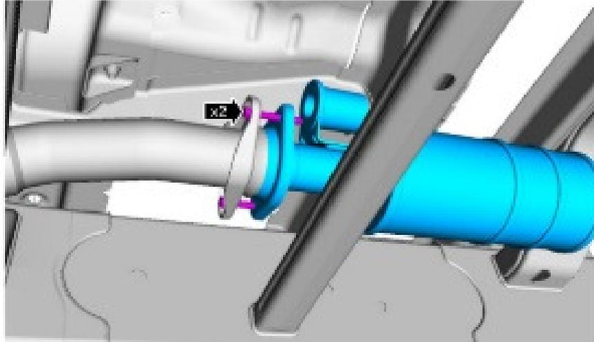
**STEP 5:** Slide the muffler and tailpipe rearward out of the isolators and then forward to remove.
