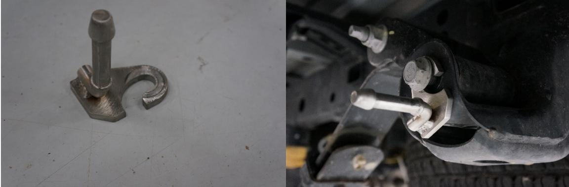
**STEP 7:** Once installed be sure to torque the shackle bolt to 235 Nm (173 lb-ft)
