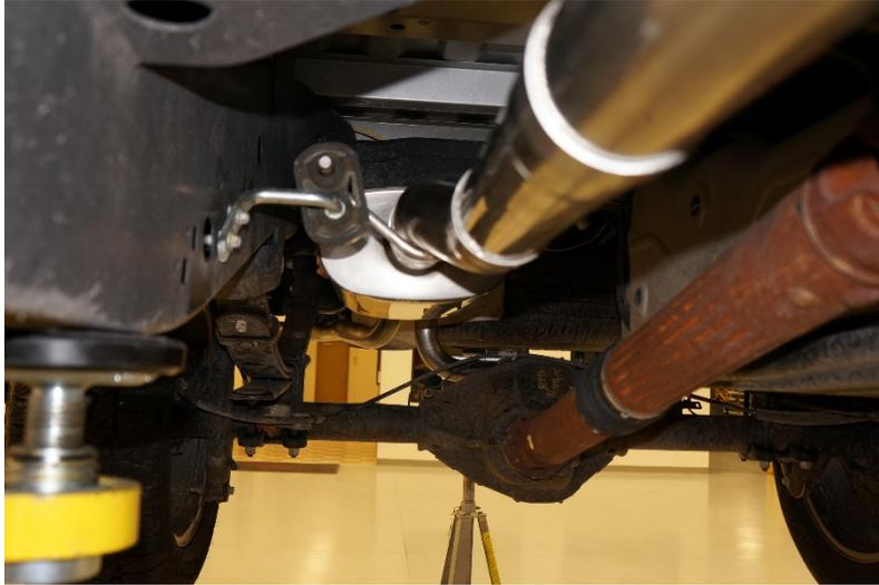
**STEP 9:** Locate the right side tail pipe, again be sure to slip the clamp onto the pipe prior to installing the tail pipe. Install one of the rubber exhaust isolators onto the hanger as shown in the second picture.
