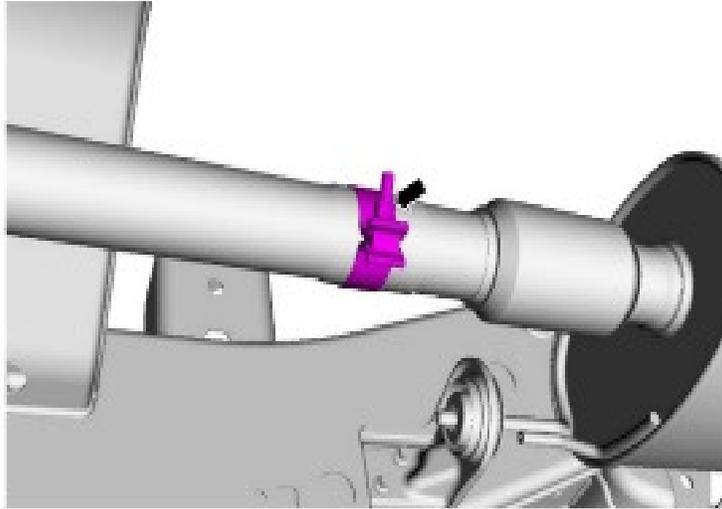
**STEP 3:** Release the locator tab out of the muffler inlet pipe.
