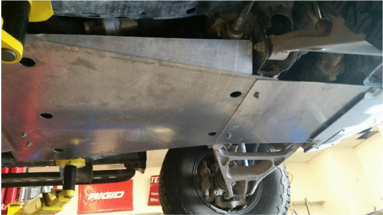
Locate the 3 small bolts provided with the kit. One is shorter and has a special short jam nut. Install the short bolt in the far right (passenger) side with the nut up. This bolt must be in the correct location so it will not rub on the wire loom that crosses over here. Put the other 2 bolts into the other 2 rear most holes.
