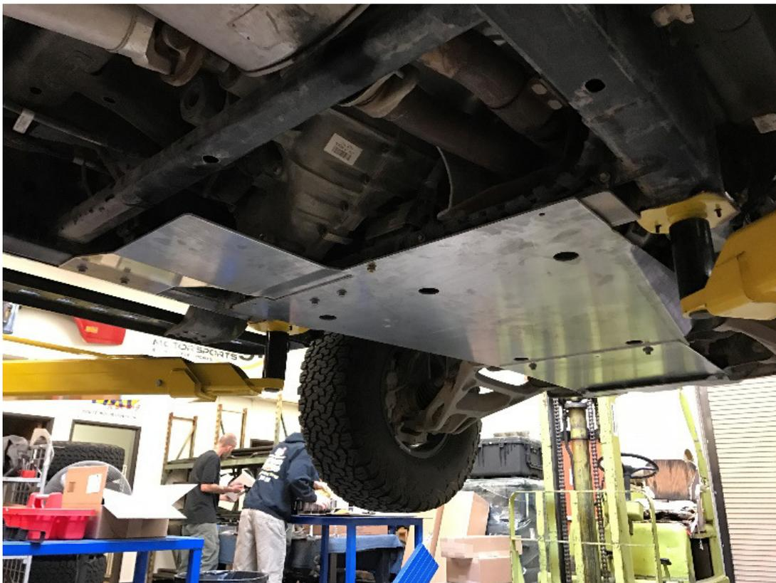
Move the large skid plate as needed until front and rear holes line up well. Re-install the factory bolts in the front section where the mid square skid plate matches up with the larger rear skid plate. Use the 2 outside holes even though this plate may have 3 holes. The center hole is left blank on this application.
