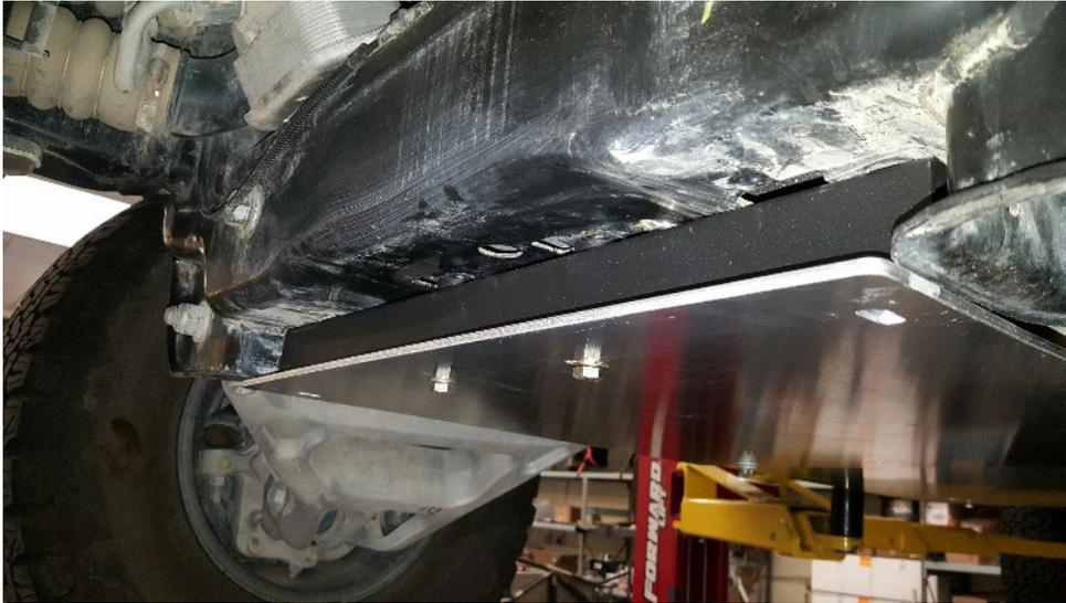
Locate the larger steel part that is installed over the transmission cross member. Remove the nuts off the transmission cross member bolts and slide the plate over the exposed bolts. Re-install the nuts with medium thread locking compound and torque to 76 lb. ft. to secure the cross member and the plate. When installing make sure the plate is aligned as it is in the photos.
