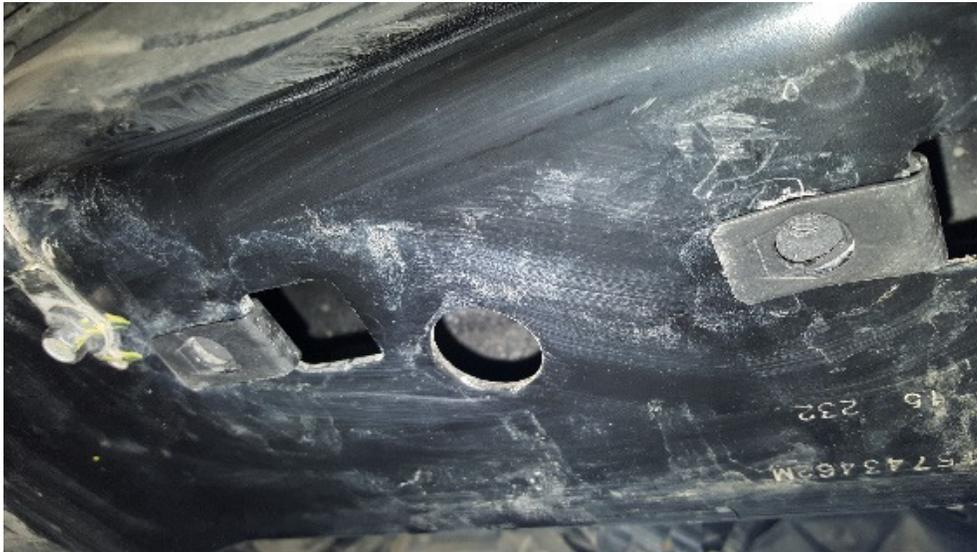
Locate the mid skid plate square section and the square tube cross member. Use the long bolts to attach the skid plate and square tube cross member. The aluminum plate has round holes and oval shaped holes. The oval holes go toward the front of the truck and these are the center holes you should use now. Put the long bolts in the 2 holes, but don't tighten yet. The square tube cross member has 2 spacers that are on the top when installed.
