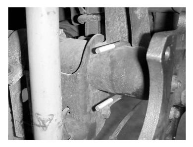
**STEP 25:** Slide the caliper brace into place over the U-bolt as shown and loosely install the nuts.
