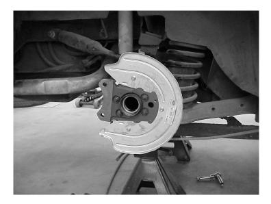
!!! Caution: Care must be taken not to let axle shaft splines damage inner wheel bearing oil seals or rear wheel bearing assembly.!!!
