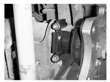
STEP 26: Install new rear rotors (Item 5) on the axle using a lug nut to temporarily hold the rotor in place.
