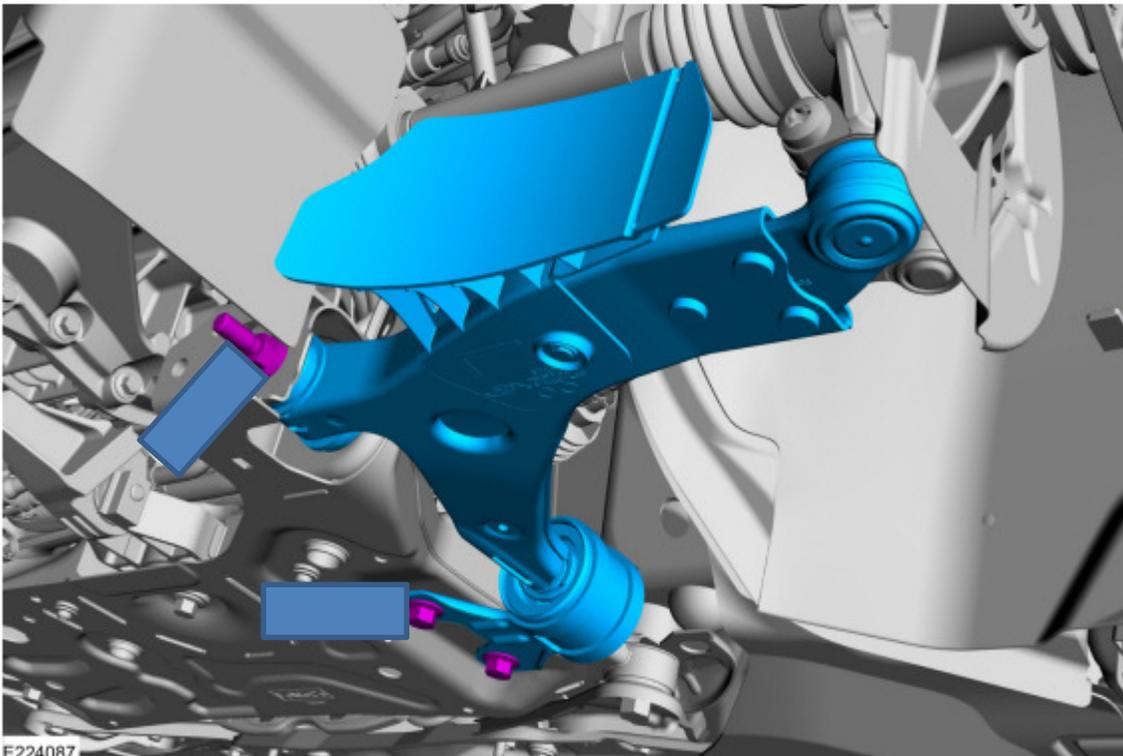
Slide deflectors onto the lower control arm.
