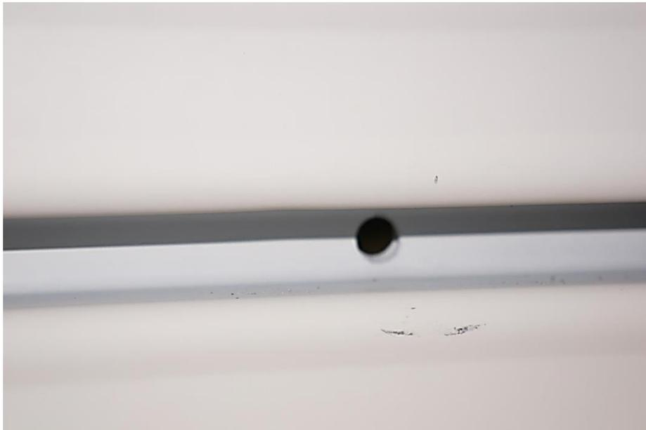
Hold Drilled through the Channel of the Front Bumper Beam
