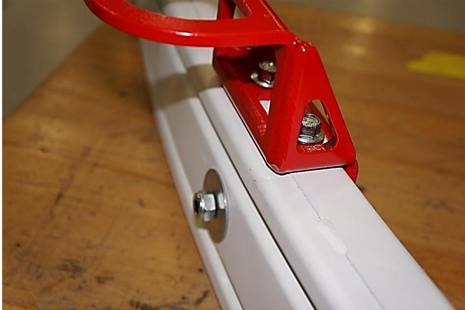
21. Bolt the Tow Ring to the Front Bumper Beam.
