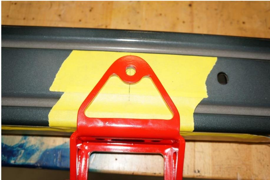
12. Set the Tow Ring on the Bumper Beam with the Back Side of the Bumper Beam facing up. Center the Hole on the center line you have drawn and mark the two (2) Bottom Bolt Holes. (picture below)
