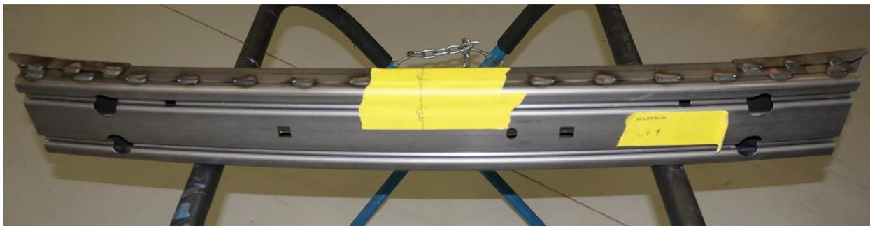
16. On the bottom of the Front Bumper Beam, find center and draw a line across the bottom then, transfer that Center Line across the Back of the Bumper Beam.
