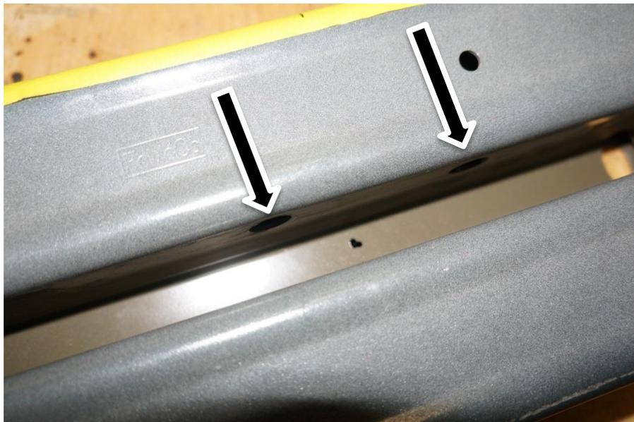
19. Fit the Tow Ring to the Front Bumper Beam temporarily to Transfer the Rear Bolt Hole Location into the channel on the back side of the Front Bumper Beam. Use the Two (2) shorter Bolts through the holes previously drilled.
