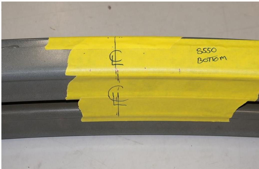
11. Find the Center of the Bottom of the Rear Bumper Beam as well as the Rearward facing side. Draw a line across both Planes.
