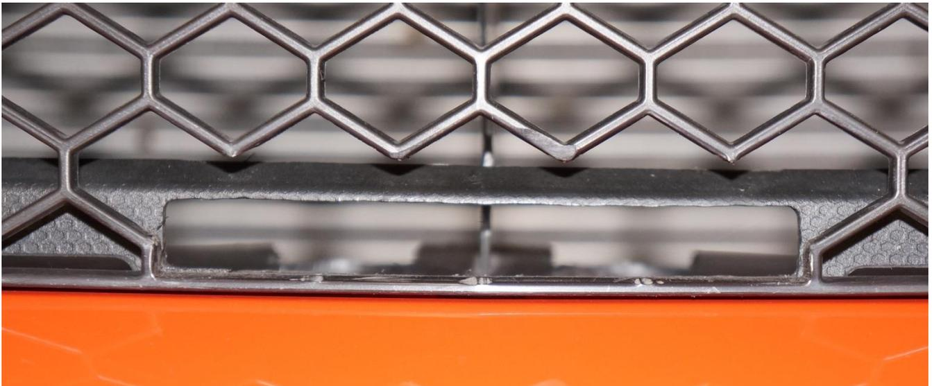
Find the Vertical Centerline of the Upper Grille. At the Bottom of the Grille, remove the Honeycomb as shown above. The section of Grille to be removed will be  $\frac{3}{4}$  inch tall by 4 Inches wide. Also, behind the Grille, notice the trim piece that is modified as well. This piece also needs to be trimmed to 4 inches wide but only as tall as necessary to leave the top and bottom in place.
