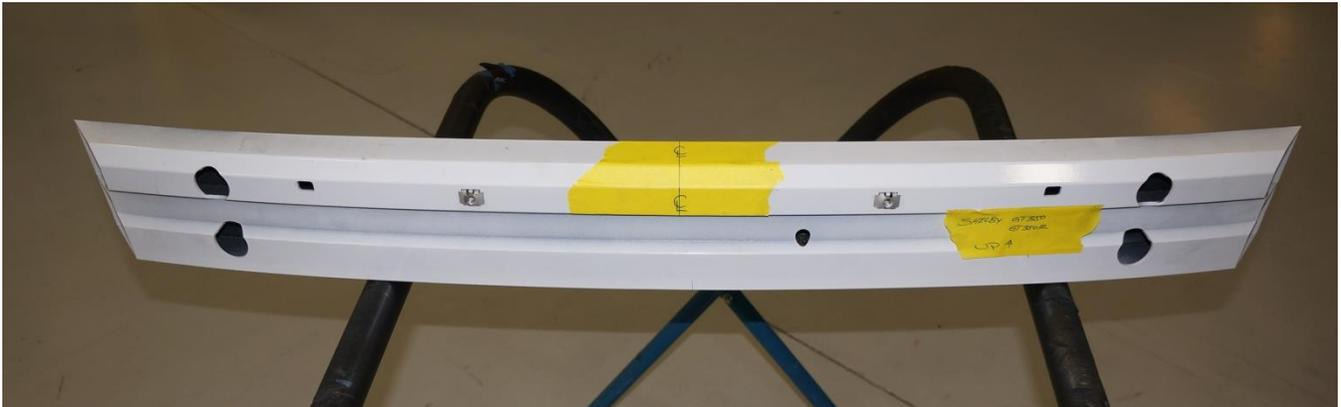
Find Center on the Bumper Beam and Mark a Line as shown above.
