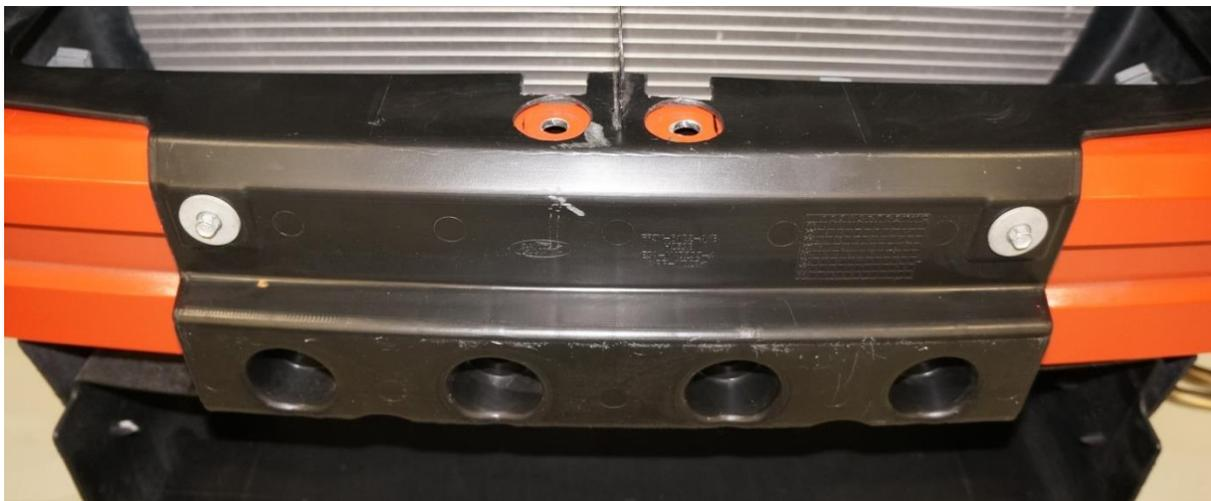
The Hole cut in the Radiator Air Deflector will allow clearance for the upper spacers and the Nut on the bottom of the Bumper Beam.
