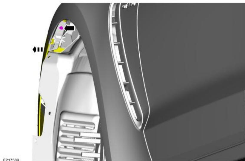
Remove the Screw and separate the Front Bumper from the retention clip on both sides
