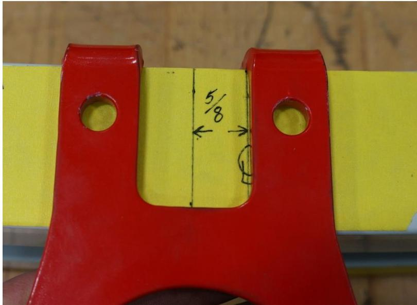
Position the Tow Ring with the Ring facing forward and the inside of the leg aligned with the Line marked 5/8 inch from the Center Line. Transfer the Holes to the Bumper Beam.
