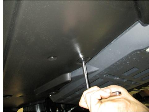
**STEP 22:** Using the bolts removed in STEP 3, install the (2) outboard bolts and torque to 15 in.-lb.
