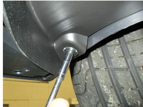
**STEP 4:** Remove the (3) rearward bolts securing the deflector.
