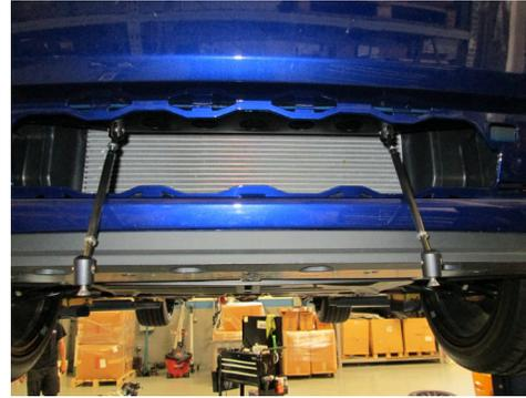
**STEP 12:** Insert the support rods through the grille openings shown below and align grille with the fascia.
