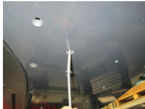
**STEP 17:** Install the splitter support rods to the splitter and torque bolts to 28 in.-lb.
