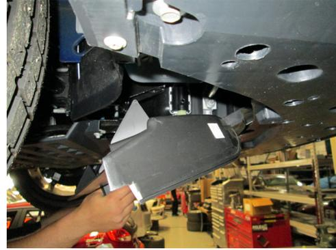
**STEP 6:** From the backside of the fascia, gently unclip the temperature sensor from the lower grille.
