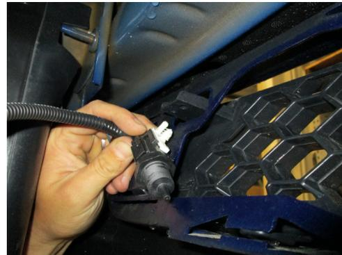
**STEP 7:** From the backside of the fascia, gently unclip the lower grille retaining clips from the fascia (12 locations). Remove the lower grille from the vehicle.
