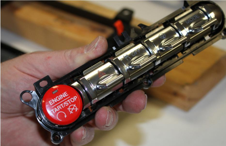
28. Reinstall the engine start and toggle switch assembly
