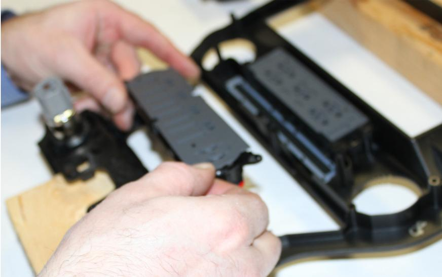
24. Remove the engine start and toggle switch contact pad
