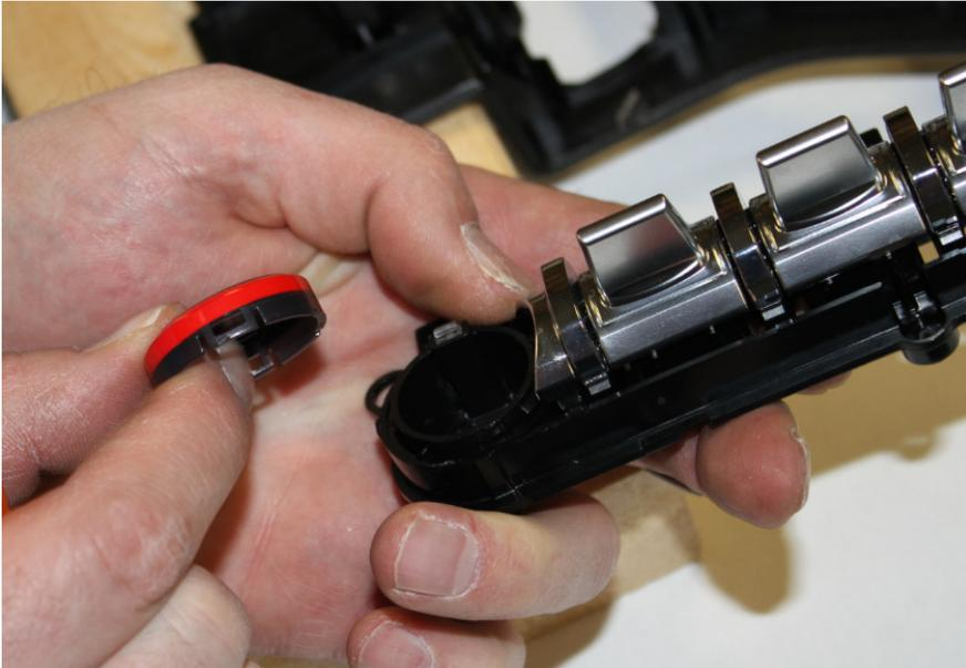
27. Gently line up the new red GT350 starter button and click it into position. Make sure that both retaining tangs are fully locked into place.
