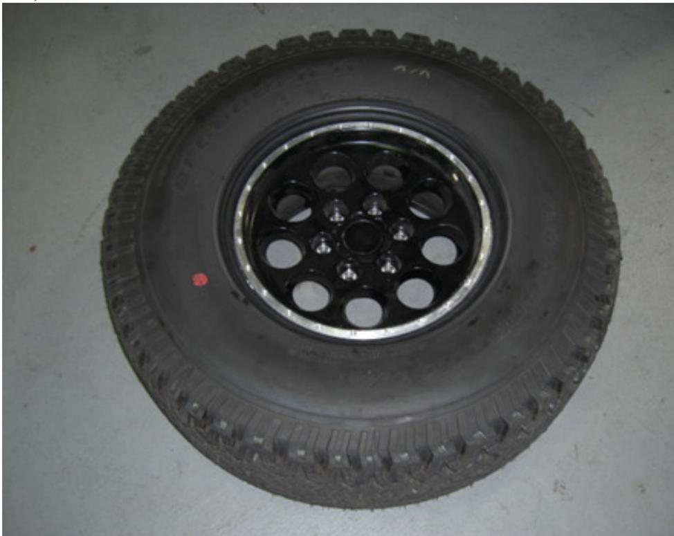
Pic 3.1 – Outer tire bead fits on wheel flange
