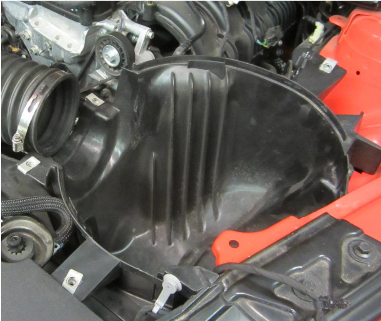
Install air bucket/air inlet assembly into vehicle. Do not bolt bucket down.
