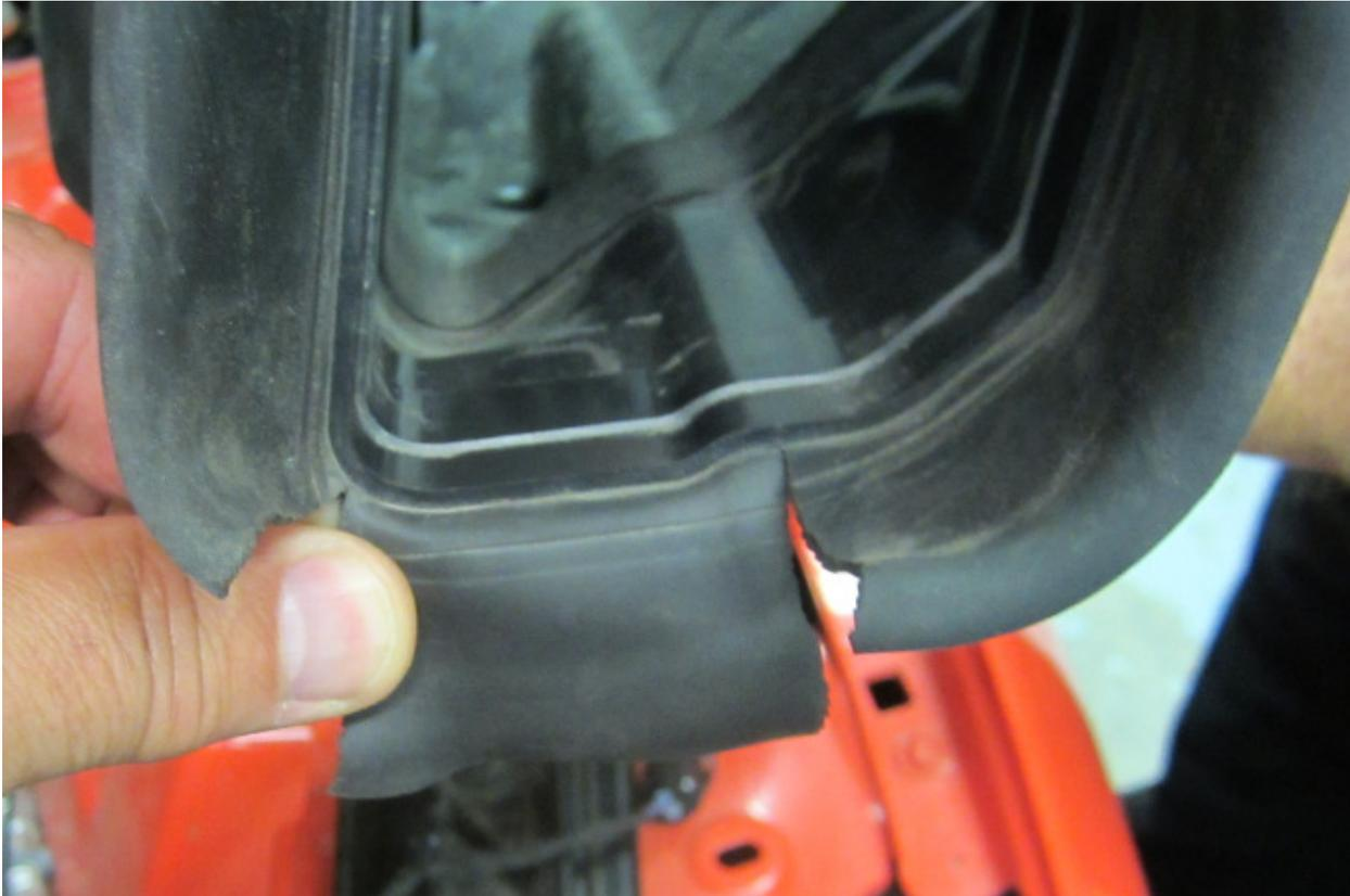
Modify air inlet by cutting rubber seal.
