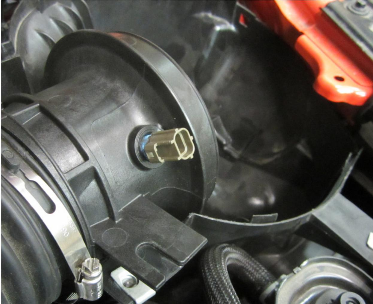
Install IAT sensor into adapter and install adapter into hose. Do not tighten clamp.
