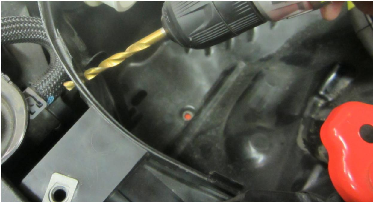
Drill hole for harness retainer.
