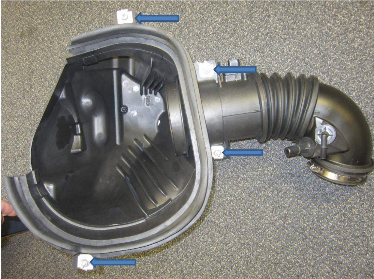
Remove air filter. Save air filter for reuse.
