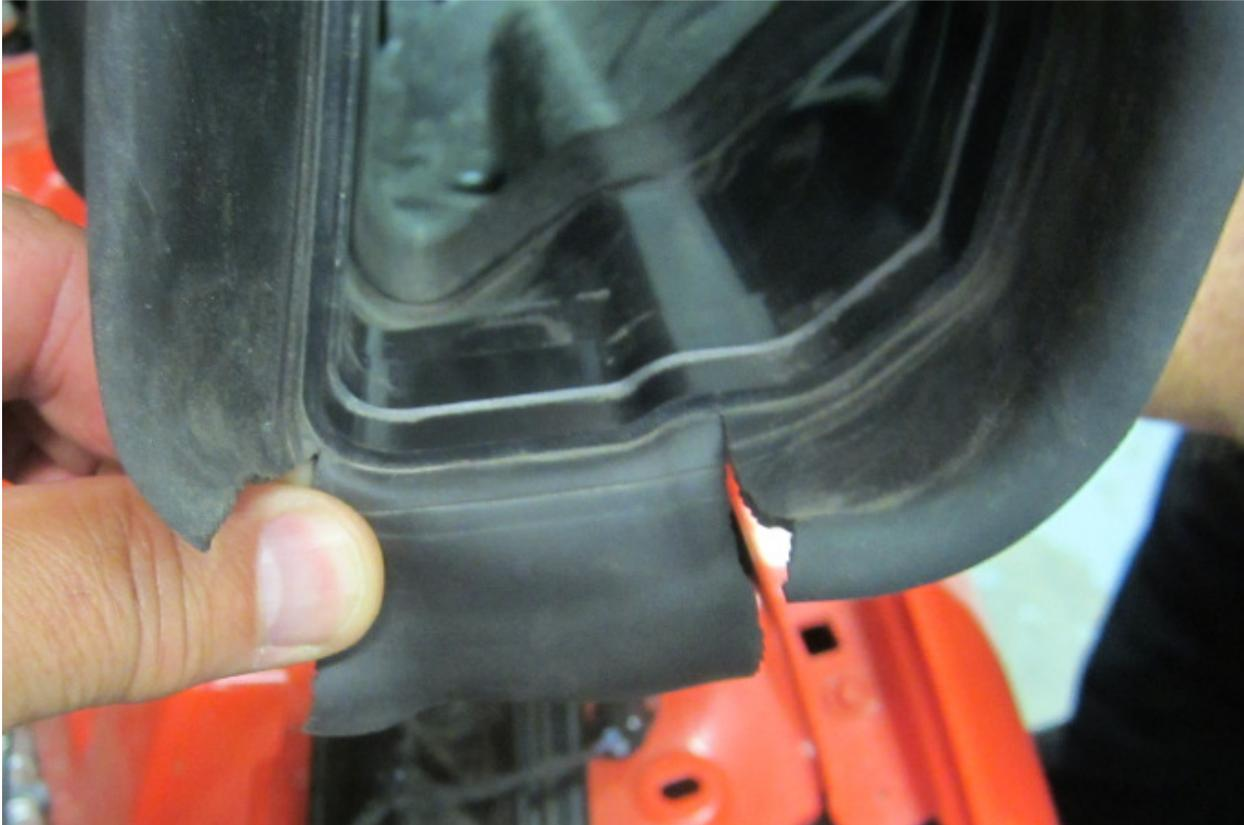
Modify air inlet by cutting rubber seal.
