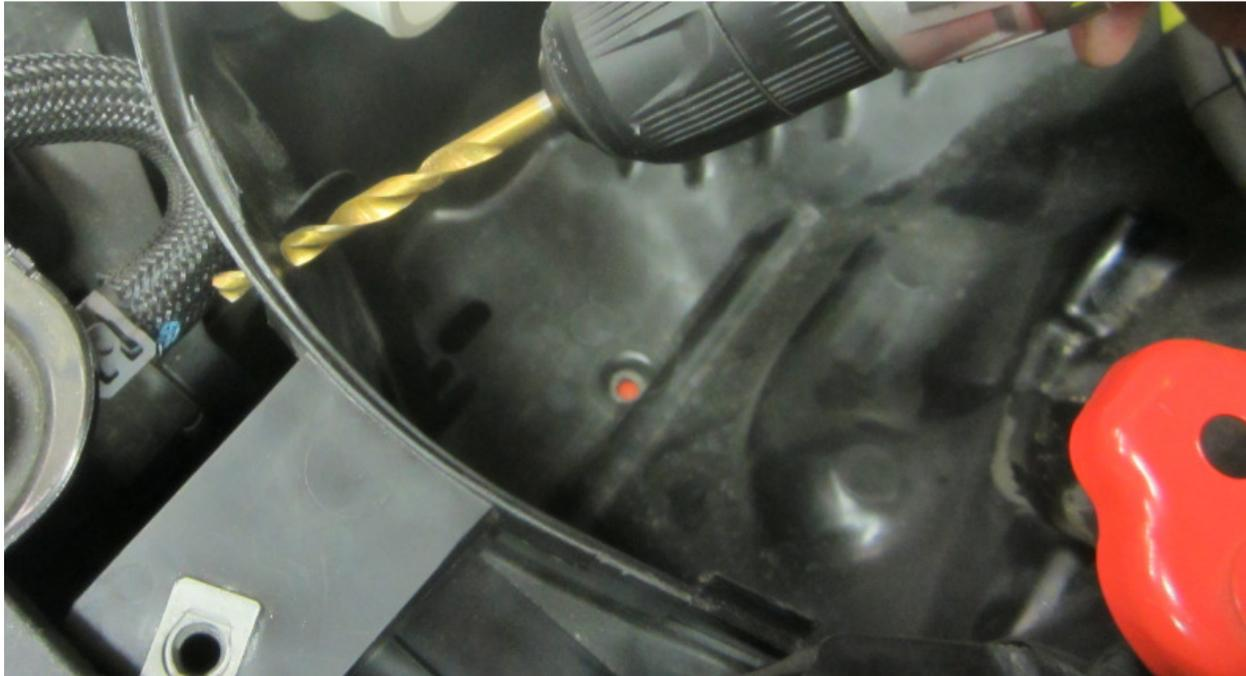
Drill hole for harness retainer.
