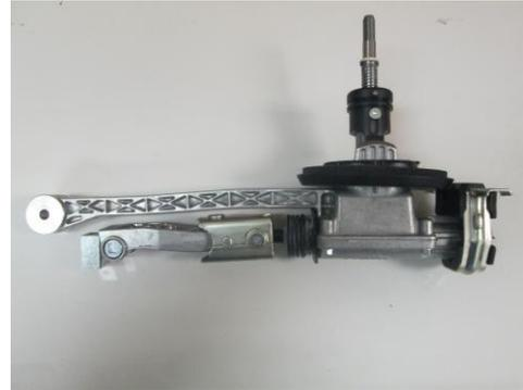
**STEP 43:** Install the gearshift lever assembly. Install the gearshift lever bolt (1). Torque: 133 lb.in (15 Nm). Install the gearshift lever-to-transmission bolt (2). Torque: 30 lb.ft (40 Nm)
