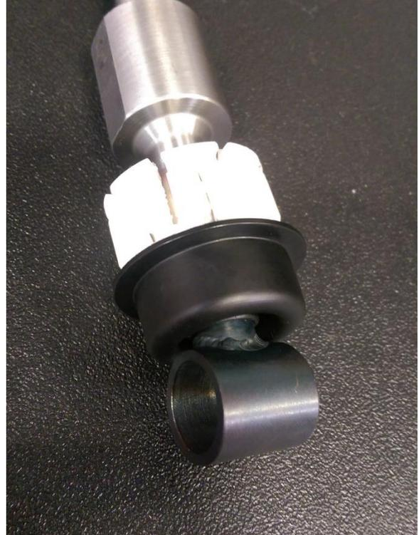
**STEP 17:** Align the shifter pivot bushing with the shifter handle, using a rubber mallet gently tap the bushing into the shifter shaft until fully seated.
