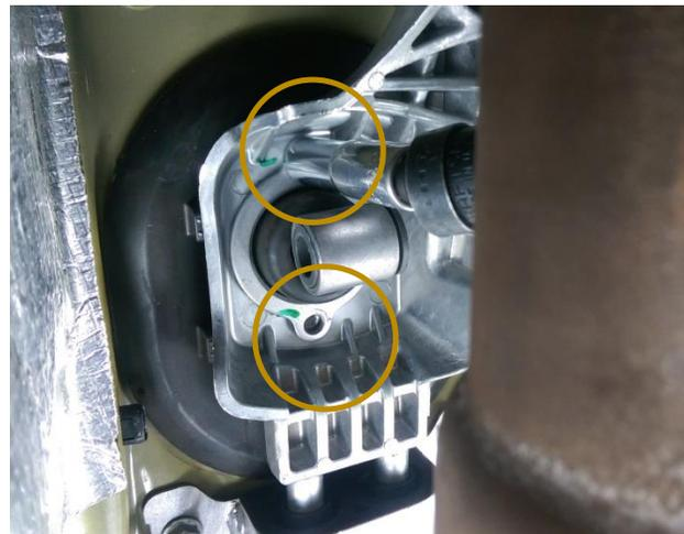
**STEP 23:** Realign the lower shifter actuation arm (3) to the new shift handle assembly. Install the steel pin (2). Install the retainer clip (1).
