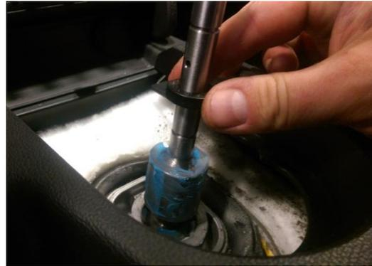
**STEP 25:** Using a small pair of pliers, carefully remove the (2) round anti-rattle pads from the OEM reverse lockout collar. Install both anti-rattle pads into the new reverse lockout collar.
