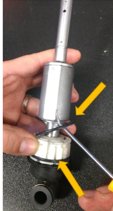
**STEP 12:** Utilizing the steel pin removed in Step 8 or a suitable punch, gently tap the shifter pivot bushing to remove from the shifter handle assembly.
