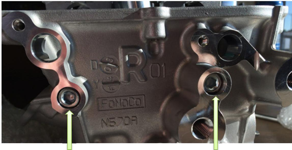
Install new pipe plugs provided and torque to 10lbf + 180deg of rotation.
