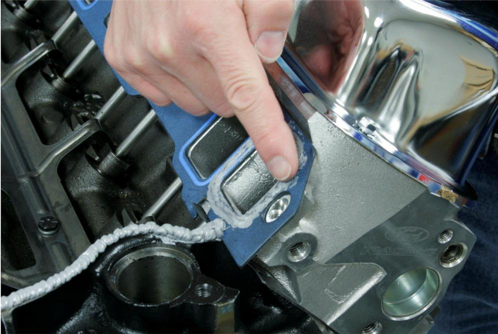
1. Set intake manifold on engine.
