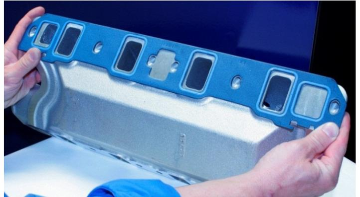
3. **Inspect intake manifold for debris, and make sure it's clean.**
