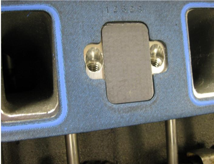
14. Rub an initial thin layer of silicone onto the end rails of the intake manifold and block.
