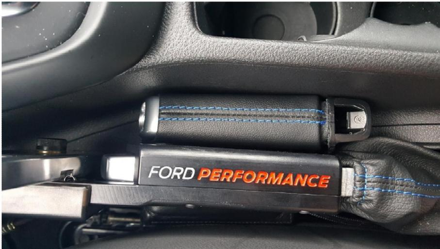
**Figure 2: Chassis and Clamshell assembled onto parking brake aluminum casting.**
