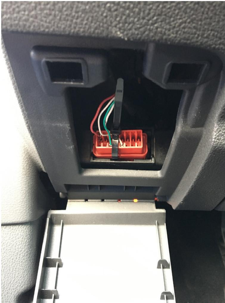
**Figure 7: OBD2 connector fully secured.**
