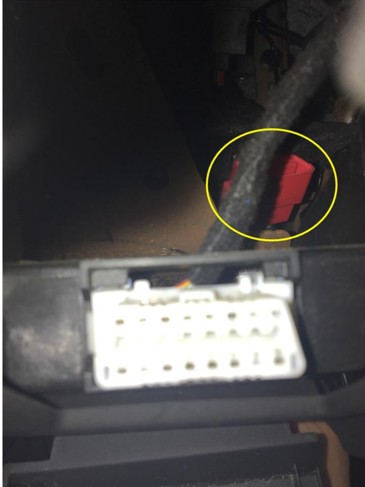
**Figure 5: Drift Stick wiring connector seen through OBD2 door during installation**
