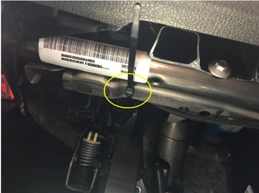
**Figure 6: Securing the wiring above the driver pedals.**
