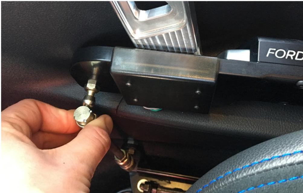
**Figure 8: Activate the quick disconnect to raise the parking brake**
