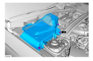
2. Loosen the nut and position the negative battery cable. *Torque*: 44 lb.in (5 Nm)
