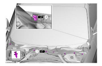
3. Lift cowl panel grill enough to access (2) bolts that retain plastic cowl extension. Wiper arms do not have to be removed.
