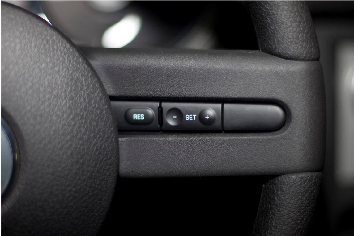
3. Once the desired launch control set point is achieved, press the "RESUME" speed control button. The in dash tachometer will again sweep to 8000 rpm, back to the desired set point, and finally back to the current engine speed (0 if the engine is off). This launch control set point is now stored in the PCM's non-volatile memory and will maintain this value until it is changed again even if the power is removed from the PCM.
